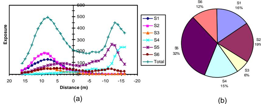
Fig. 4; (a) Ensemble average exposure profiles of a pedestrian crossing south Gloucester place from D to A. The exposure profiles are obtained by averaging 14 instantaneous exposure profiles which take place immediately after the favourable light (the green man) is switched on. Total is the exposure profile due to the combination of S1, S2, ..., and S6. Negative – D, positive – A. (b) Percentage contributions of the six sub-sources to the integrated exposure of a pedestrian crossing D → A.
