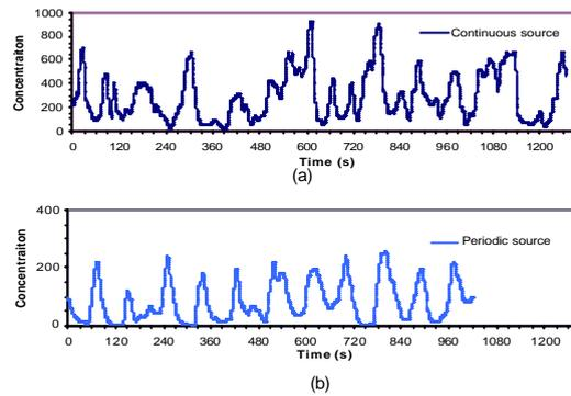
Fig. 2; Concentration time series at the middle point of A—D (Fig 1(a) (b)) at pedestrian level. (a) – continuous source, data from the simulation for six sub-sources; (b)– periodic source with period of 90s, data from the simulation described the last paper (Wang et al., 2005).
