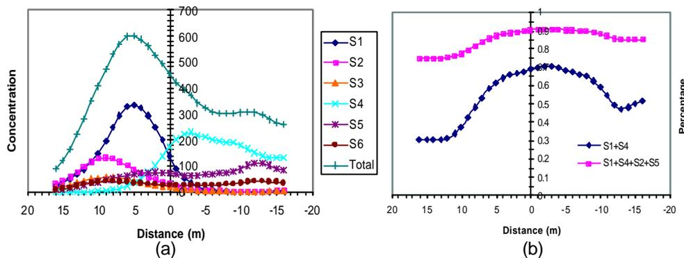
Fig.3 (a) Distribution of average concentration along the crossing route A -D. – Negative D, Positive – A. Total is the sum of concentration due to all 6 sources. (b) Contribution in percentage of the average concentration along the crossing route A -D.
