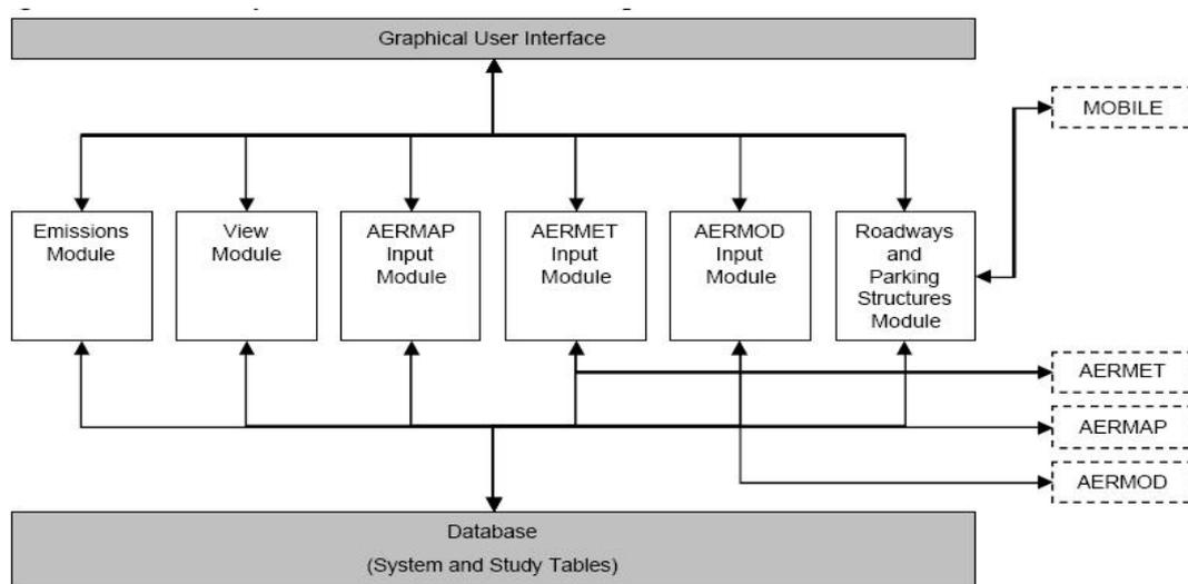
*Fig. 1; EDMS system architecture and components.*
