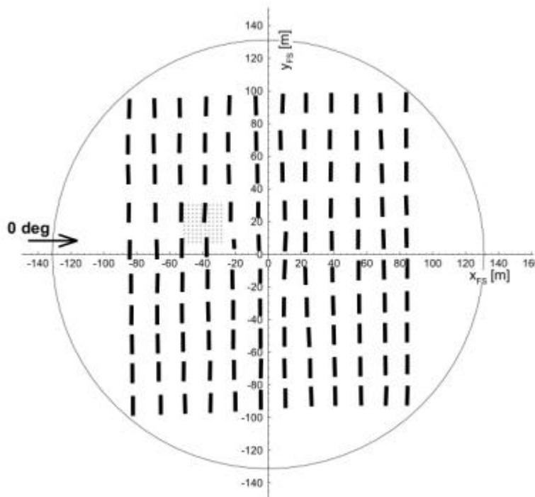
Fig. 1; Array of obstacles (MUST) and the fine measuring grid.
