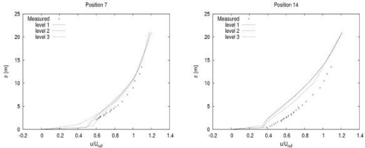
Fig. 1; The  $u/U_{ref}$  velocity profiles at two different positions from the  $0^\circ$  case.
