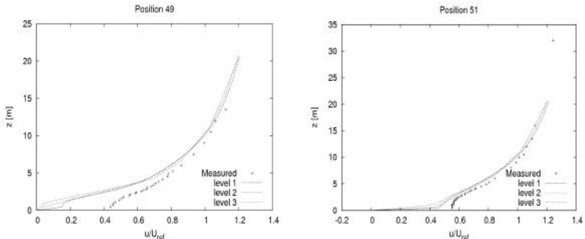
Fig. 2; The  $u/U_{ref}$  velocity profiles at two different positions from the  $45^\circ$  case.
