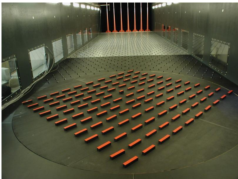
*Fig. 3; The MUST wind tunnel model inside the large wind tunnel of Hamburg University.*
