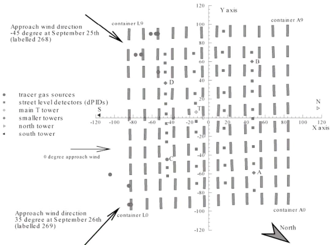
Fig. 2; The MUST field campaign: sketch of the experiment layout.
