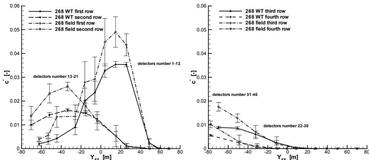
Fig. 5; Comparison of the MUST field (depicted by the squares and diamonds) and wind tunnel (depicted by the triangles) mean dimensionless concentration for the trial 2681849 (-41° wind direction and source no. 29). The first and second row of detectors ( $x=-50$  and  $-10$ , respectively, see Fig. 2) is shown in the left chart, the third and fourth row of detectors ( $x=16$  and  $45$ , respectively) is shown in the right chart.
