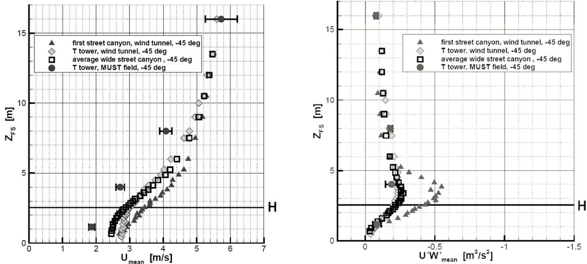
Fig. 4; The vertical profiles of the mean wind speed (left chart) and the vertical momentum flux (lower chart) for  $-45^\circ$  approach wind direction.
