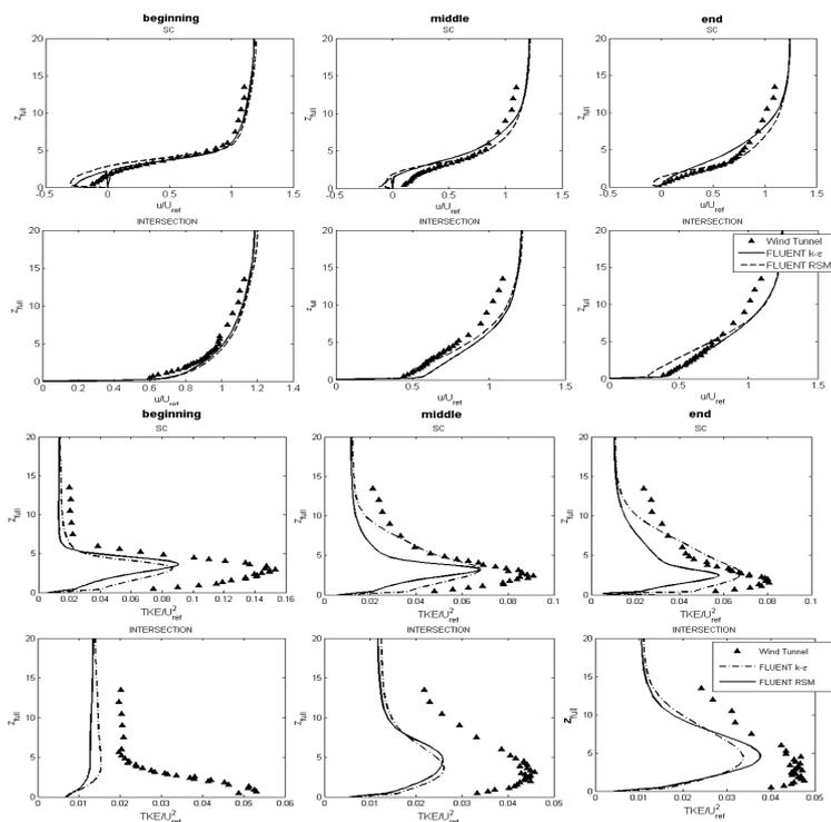
Fig. 2; 0° approaching flow case: vertical profiles of  $u/U_{ref}$  (top) and  $TKE/U_{ref}^2$  (bottom).
