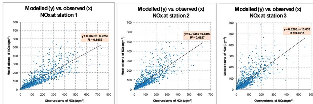
Figure 4. Scatter plot of observed (x) vs. model calculated (y) concentrations of NO<sub>x</sub> at station 1 (left), 2 (middle) and 3 (right). All hourly values (N = 1345) with wind direction towards the stations 1-3 between 1 January 2002 and 15 April 2002 plotted.
