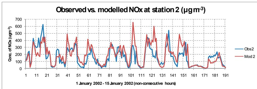
Figure 2. Time series plot of observed and model calculated concentrations of  $\text{NO}_x$  at station 2 for the first half of January 2002. This was a period with (strongly) stable conditions ( $\max \Delta T_{10-2m} = 4.0$  at hour 132) with low wind speed (min  $U_{10m} = 0.1 \text{ ms}^{-1}$  at hour 40).
