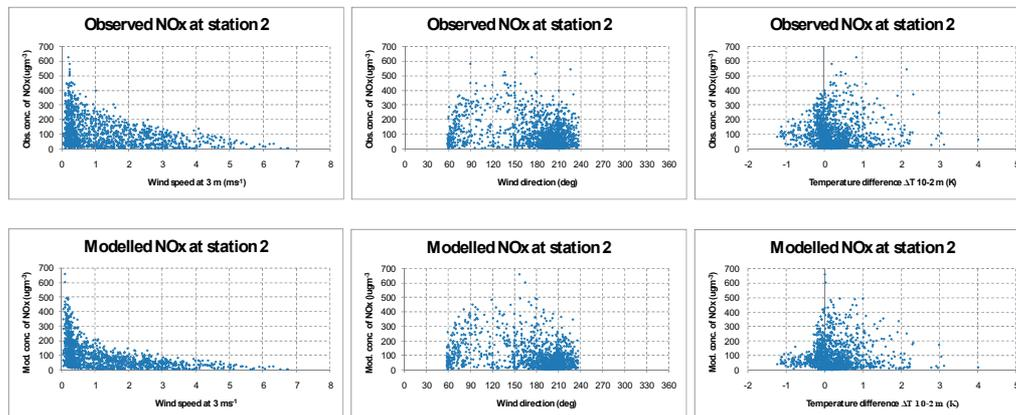
Figure 3. Observed (top row) and model calculated (bottom row) concentrations of NO<sub>x</sub> at station 2 as a function of wind speed at 3 m above ground (left), wind direction (middle) and temperature difference between 10 and 2 m indicating stability (right). All hourly values (N = 1345) with wind direction towards stations 1-3 between 1 January 2002 and 15 April 2002 plotted.
