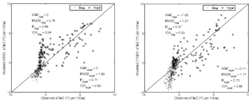
Figure 2. Observed and modelled vertical temperature gradient at Järnbrott mast site from TAPM and MM5 respectively. The results are based on hourly data of near-surface and 105-m measurements/simulations during the period from 7–19 May 2001. The temperature gradient during night hours (20:00–07:00 UTC) is denoted by square to show nocturnal temperature inversion for clarity. Statistical parameters at day and night are presented within the plot.
