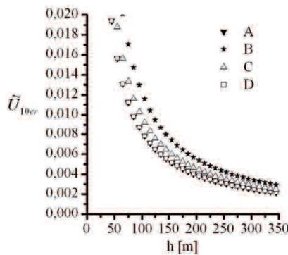
Figure 1. The dependence of the critical speed  $\tilde{U}_{10cr}$  on the source height  $h$  at different stability classes for rural region.
