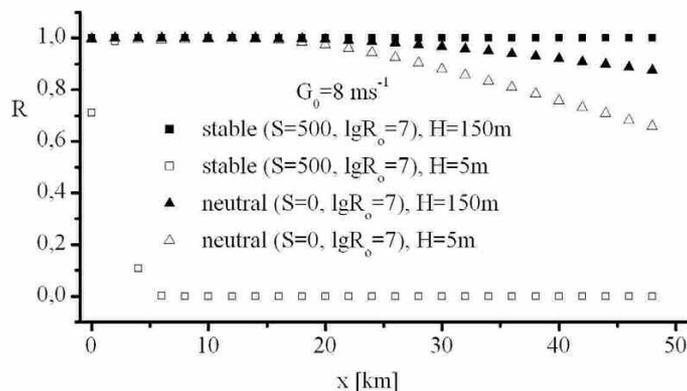
Figure 4. Dependence of wind rotation effect on the distance from the source  $x$  for plume surface concentration characterized by the dimensionless number  $R(x)$ ,  $R=1$  without rotation,  $R \neq 1$  with rotation.
