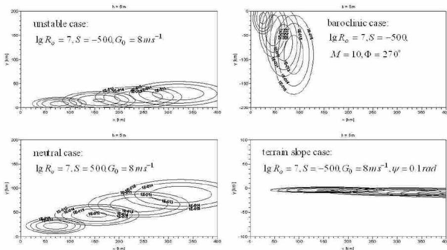
Figure 3. Isolines of surface cloud concentration  $c(x,y,0,t)$  in moments  $t=3, 6, 9, 12$  h, for different PBL turbulent regimes and  $h=5$  m. The isolines of the terrain slope case are the same as for the rest cases on the figure.
