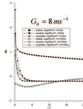
Figure 2. Plot of the vertical skewness  $Sk$  for stable ( $S=500$ ), neutral ( $S=0$ ) and unstable ( $S=-500$ ) stratification from surface source with height  $h=5$  m.
