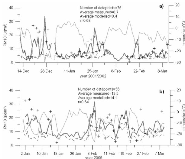
Figure 3. Comparison of measured (+) and modelled (grey solid line) daily mean concentrations of PM10 ( $\mu\text{g}/\text{m}^3$ ) at Lycksele/Sweden for two different time periods. Grey broken line is background concentrations and thin grey solid line is daily mean temperature. (a) Time period 20011214-20020310, (b) Time period 20060101-20060310.
