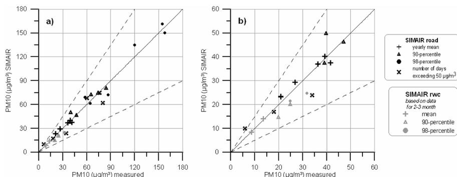
Figure 4. Comparison of measured and modelled concentrations of PM10 ( $\mu\text{g}/\text{m}^3$ ) expressed in terms of air quality levels defined by the Swedish legislation and the EU directive on air pollution levels for PM10. Broken line shows the modelling uncertainty of  $\pm 50\%$  defined for annual averages of PM10. (a) All data, (b) data below  $60 \mu\text{g}/\text{m}^3$ . The figures present the same results as given in Table 2.
