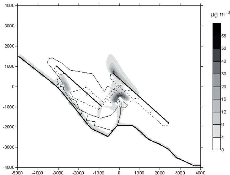
Figure 4. Forecasted daily average  $\text{NO}_x$  concentration distribution at Ferihegy Airport when the wind blows from south.
