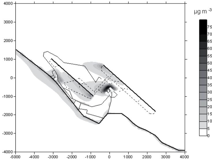
Figure 5. Forecasted daily average NO<sub>x</sub> concentration distribution at Ferihegy Airport when the wind changes direction during the day.
