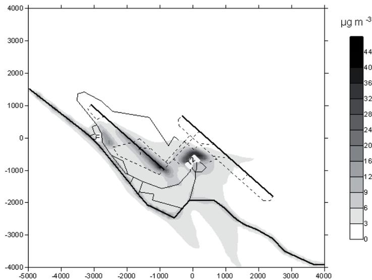
Figure 3. Forecasted daily average  $\text{NO}_x$  concentration distribution at Ferihegy Airport when the wind blows from northwest.
