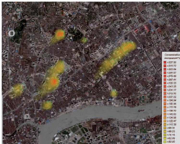
Figure 2. AERMOD Modeling Output  $\text{PM}_{10}$  ( $\mu\text{gm}^{-3}$ ) from several construction sites (green line): is possible to see, the sum effect, in terms of dust pollution from different emission sources.
