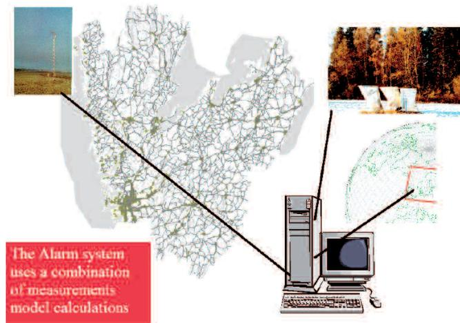
Figure 1. The ALARM-system area located in southwest Sweden. Measurements are collected once per hour and regional prognosis once every 6<sup>th</sup> hour. The area size is around 200 x 250 km.
