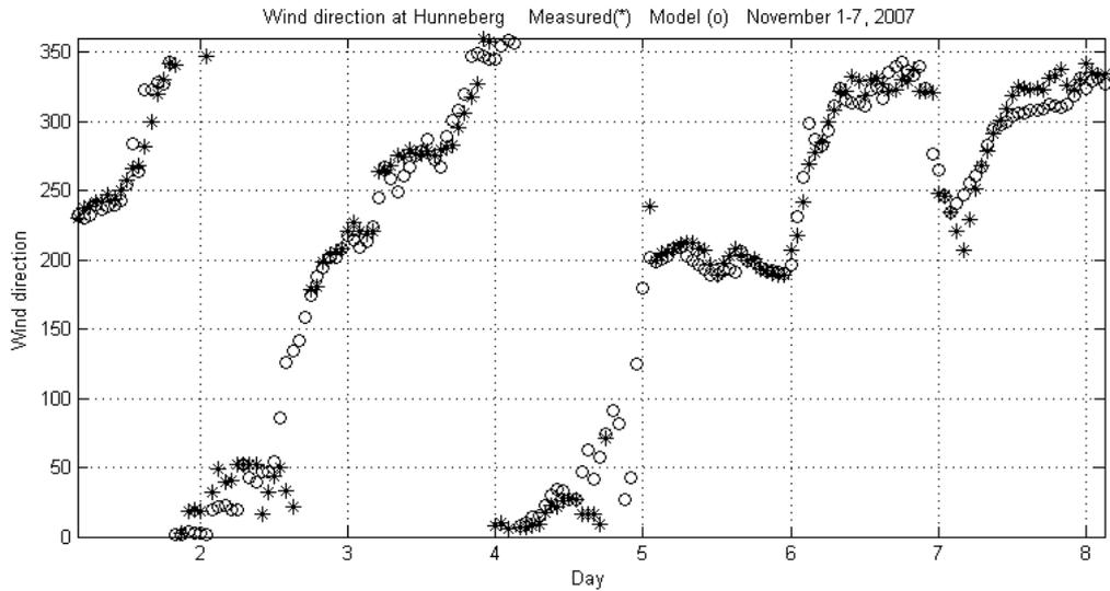
Figure 2. Measured (sodar (\*)) and simulated (o) wind directions at site Hunneberg at 175 m.
