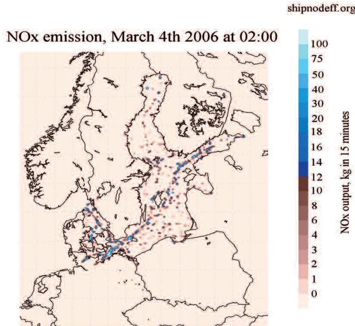
Figure 1. NO<sub>x</sub> emissions of ship traffic in the Baltic Sea area during one 15-minute period on March 4th 2006.
