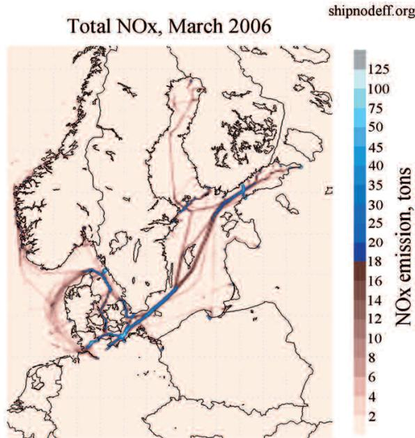
Figure 2. Total NO<sub>x</sub> release of ship traffic during March 2006.
