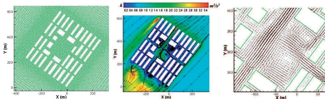
Figure 2. Structured grid (left) and calculated flow fields (middle & right) over the Piraeus domain for 08/05/2002:11:00 LST. The color map represents calculated TKE values.
