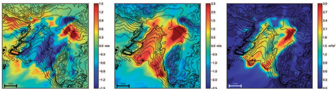
Figure 4. Difference map of the calculated average wind velocities on the first (left) and second (middle) computational layer, and average TKE on the second computational level (right).
