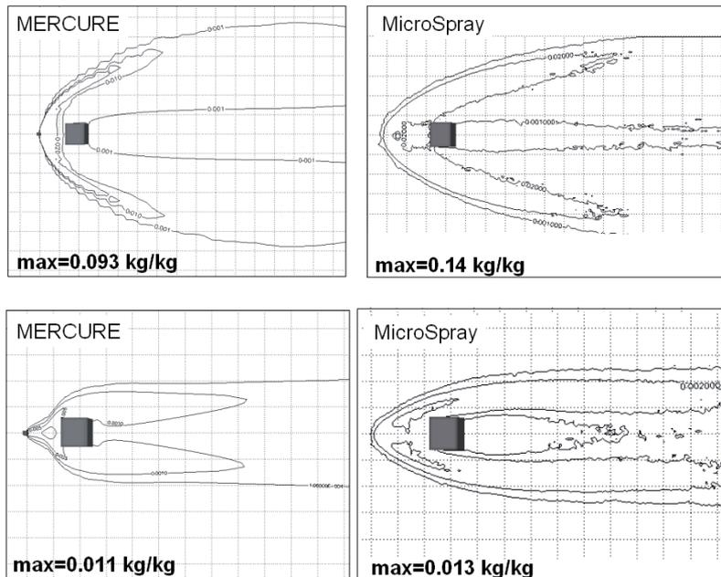
Figure 4. Glc obtained by Mercure and MicroSpray (MSS) in lower (above) and higher (below) wind speed.
