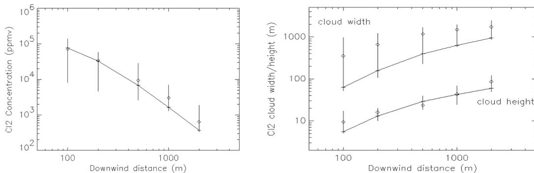
Figure 1. MSS results compared to the Macdona accident simulations from six widely-used models (from Hanna, 2007). Continuous lines indicate present results, the vertical bars show the variability (max, min) of the six models and circles locate the median of these models. Left graph refers to the Cl<sub>2</sub> concentration versus distance; right graph plots Cl<sub>2</sub> cloud width and height, both to the model-simulated concentration of 20 ppm versus distance.
