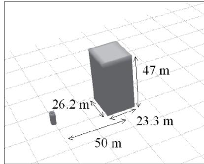
Figure 3. Plot of the dispersion situation simulated by Mercure and MicroSpray (MSS), in which the dimensions of the stack and obstacle are shown.
