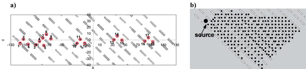
Figure 1. Measurement positions for the -45 degree case. a) towers for velocities, b) concentrations. Wind blows from the left.
