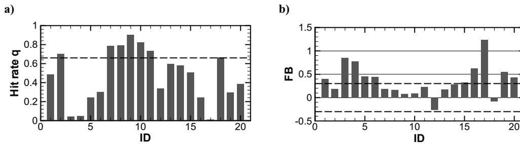
Figure 3. Metrics for the turbulent kinetic energy  $k/U_{ref}^2$  at the towers for the  $-45$  degree case. a) Hit rate  $q$ , b)  $FB$ .
