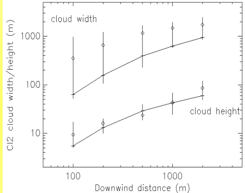
Left graph refers to the **Cl2 concentration versus distance**; right graph plots **Cl2 cloud width and height**, both to the model-simulated concentration of 20 ppm versus distance
