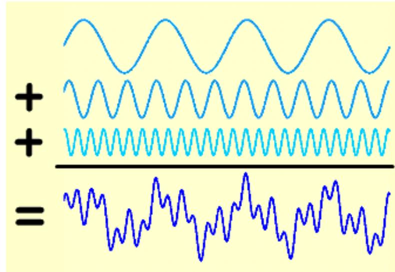
a time series  $X_t$  of length  $N$  is presented as a linear combination of harmonic functions with frequencies  $\{f_j\}$  and amplitudes  $\{A_j\}$  and  $\{B_j\}$ :
