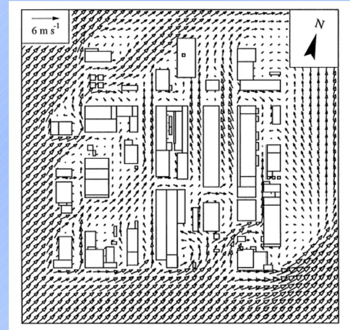
Comparison between measurements and numerical simulation
