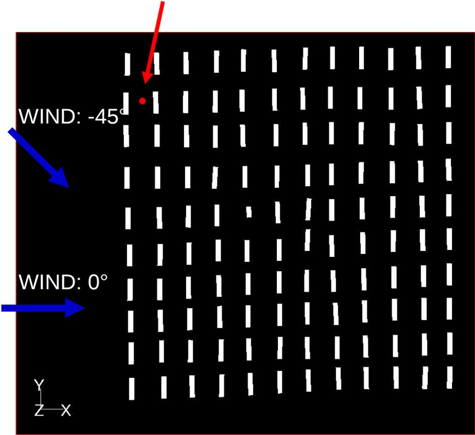
*Schematic view of the MUST building array and cases considered. The point source is positioned along the axis of the first street canyons line*
