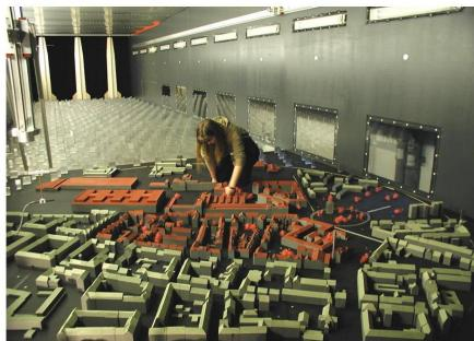
Fig. 2: Physical model of the site in the Boundary Layer Wind Tunnel of Hamburg University
