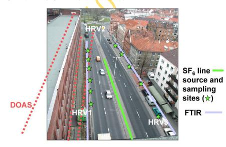
Fig.1: Street Canyon 'Goettinger Strasse with instrumentation. The picture shows the continuous monitoring stations HRV1 to HRV3 in white and the SF6-line-source at the median strip plus the sampling bag locations in green colour. The path-averaged measurements are indicated by the blue solid (FTIR) and red dotted (DOAS) lines.
