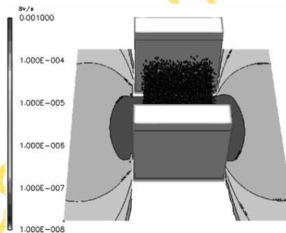
Figure 7: Influence of buildings on the gamma dose rate. Domain: 100 m x 100 m x 200 m
