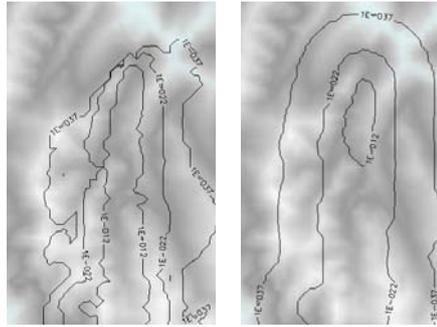
Figure 6 : Influence of the topography on the gamma exposure at ground level.
