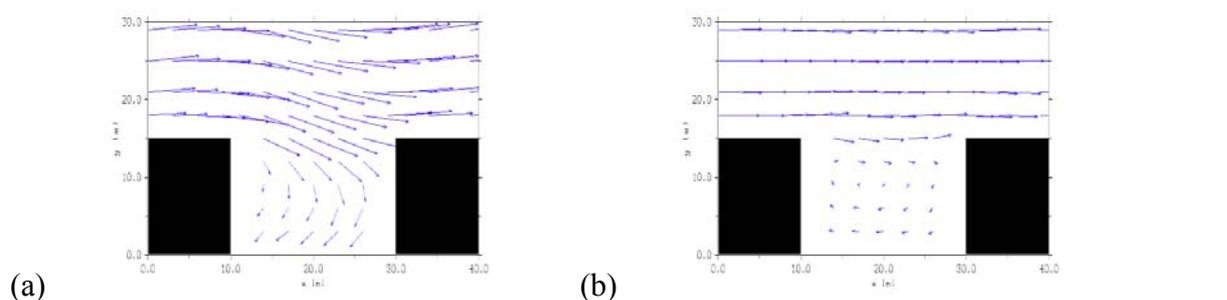
Figure 4. Horizontal wind vectors within an array of buildings. (a) wind tunnel data, (b) MISCAM results.
