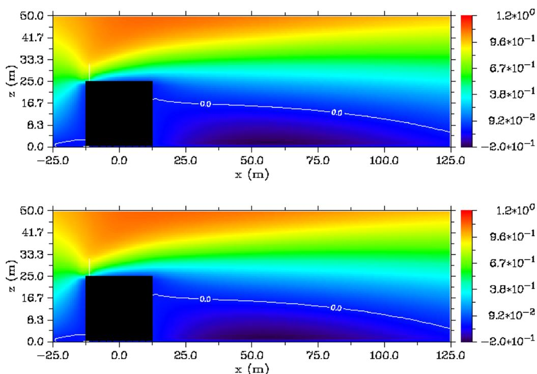
Figure 1. Wind component  $u$  (m/s) for two-dimensional flow over a beam. (above) Stationarity criterion of MISCAM applied, (below) number of time steps doubled.
