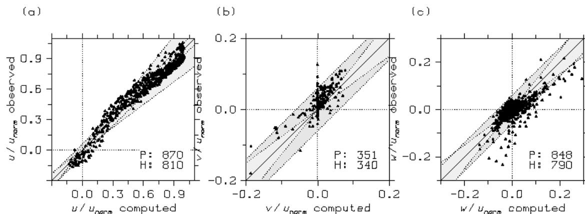
Figure 2. Computed vs. observed normalized wind component  $u/u_{norm}$  (a),  $v/u_{norm}$  (b) and  $w/u_{norm}$  (c) for flow around a cube.  $u_{norm}$  is the undisturbed inflow velocity.
