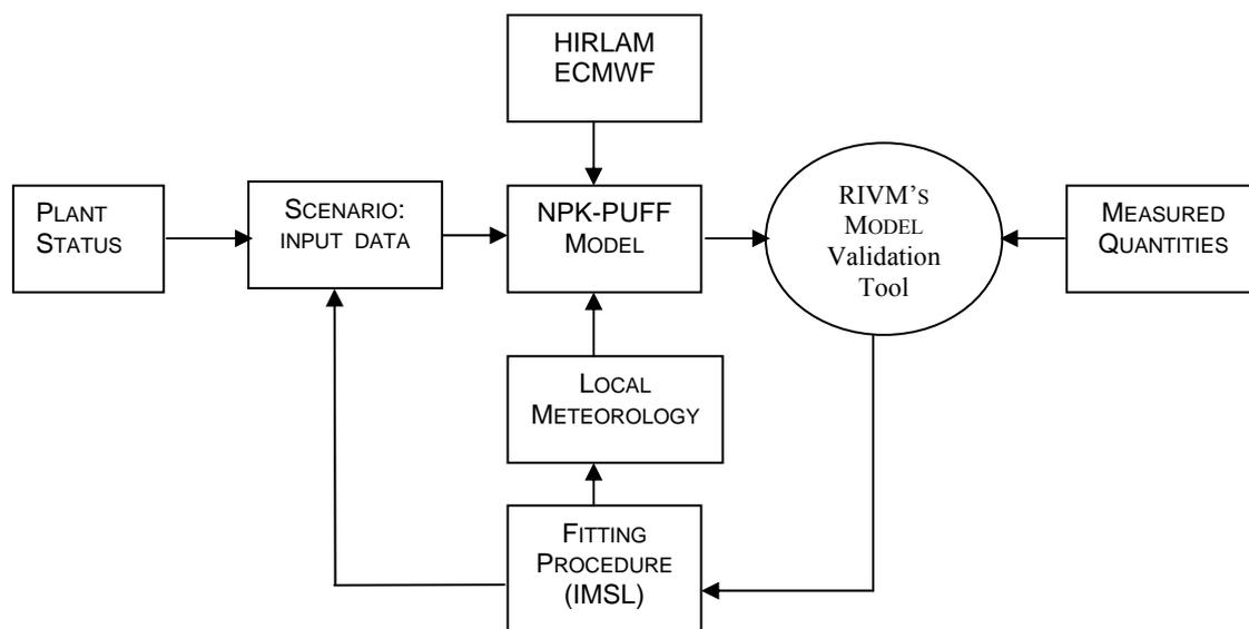
Figure 6. Flow chart of the data assimilation technique using RIVM's Model Validation Tool and a fitting procedure of IMSL to establish an improved prognosis of the dispersion modelling.
