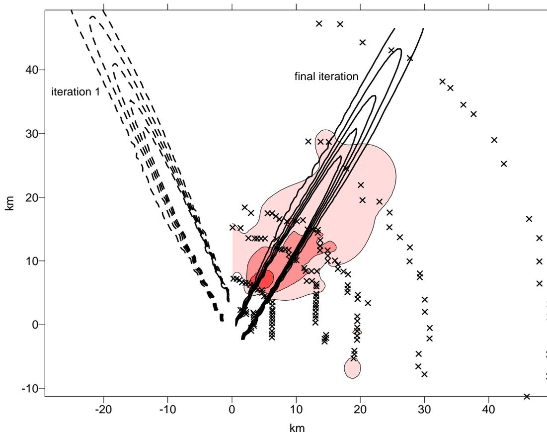
Figure 8. Graphical representation of the result from the fitting procedure for Kincaid day 1980-07-25, see also Figure 2. The crosses represent the receptor points, the filled contours show the interpolated observed concentrations, and the other contours are the modelled results of the first and last iteration.
