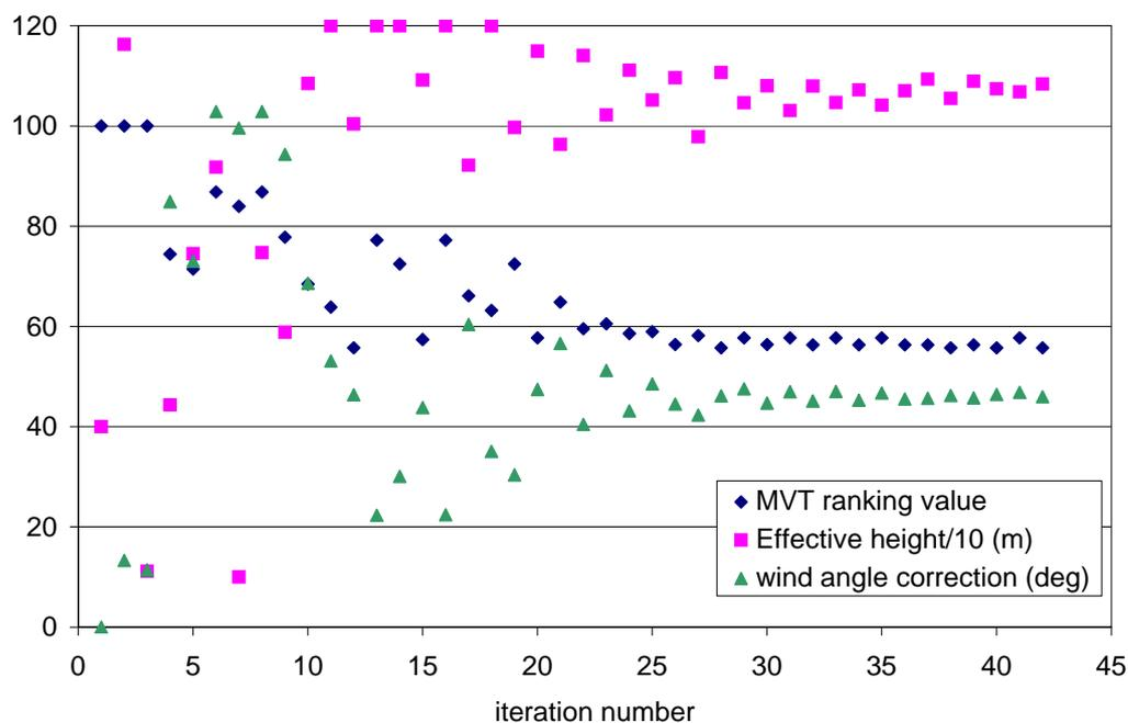
Figure 7. Results of the data assimilation technique for Kincaid day 1980-07-25, using the original input data at the start, the MVT tool and the fitting procedure. Only the effective emission height and the wind vector were adjusted.
