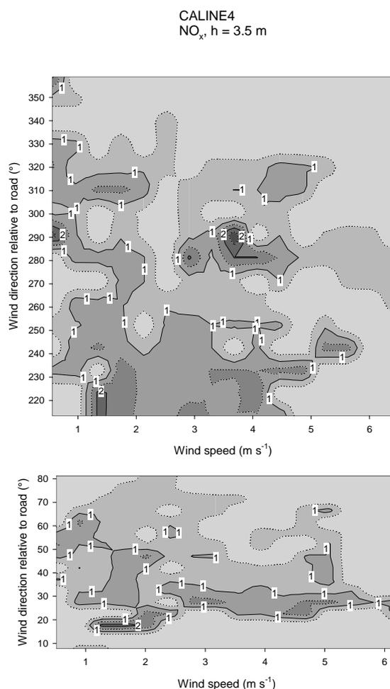
Figure 3. The ratio of predicted to observed concentrations plotted against wind speed and direction, for the CALINE4 model. We have utilized the data from both the measurement van #1 and the cabin, both of these at a height of 3.5 m.
