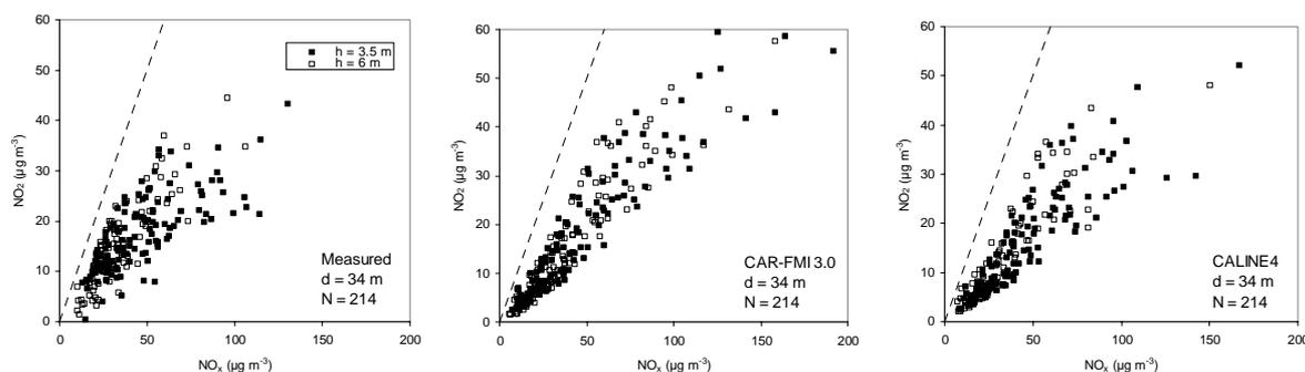
Figures 2a-c. The dependency of NO<sub>2</sub> concentrations on NO<sub>x</sub> concentrations, for the measured and predicted results at a distance of 34 m. The upper limit of NO<sub>2</sub> concentration is shown by the 1:1 line. Left panel: measured data, middle panel: CAR-FMI model, right panel: CALINE4.
