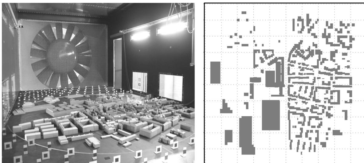
Figure 1. Picture of the physical model in the wind tunnel (left), and horizontal sketch of the obstacle representation in the numerical model (right).
