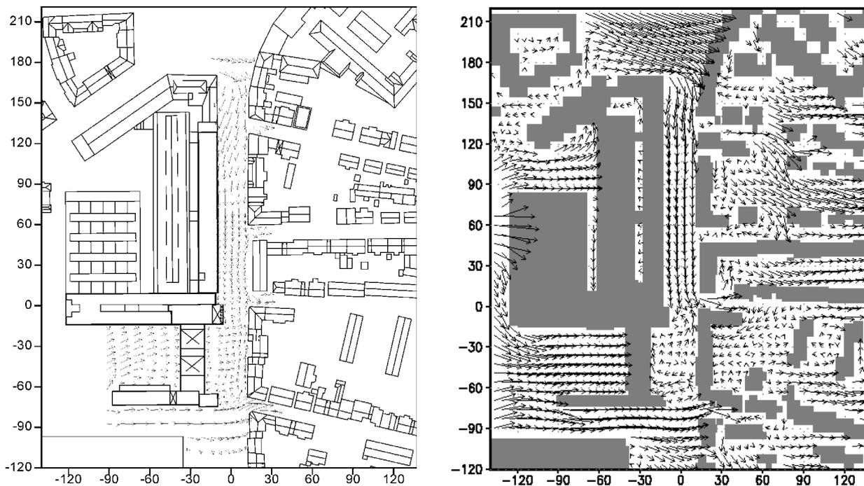
Figure 2. Flow patterns for test case 270° at 10 m above ground for wind tunnel data (left) and numerical model result (right).
