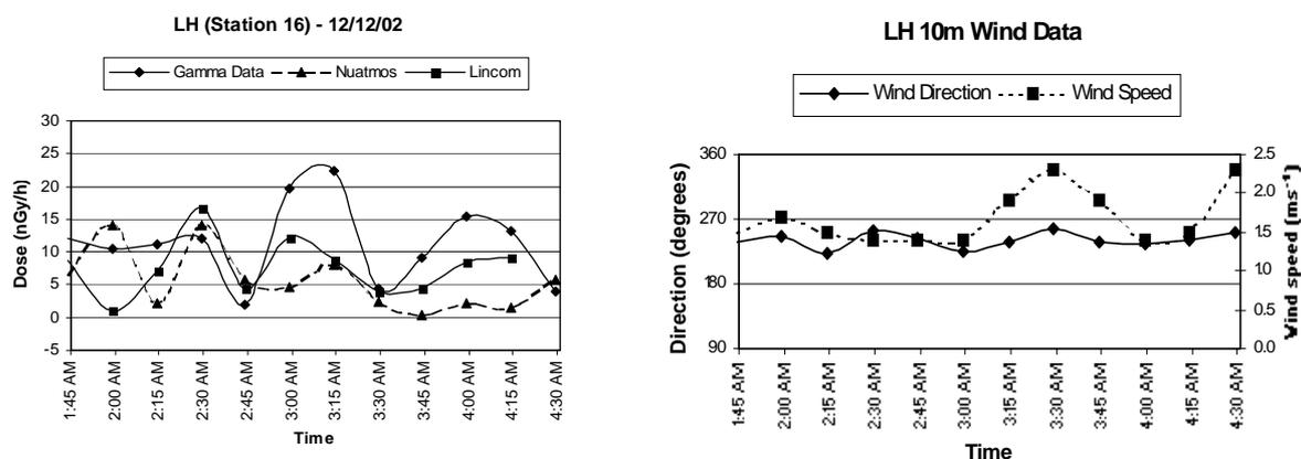
Figure 2. Examples of gamma radiation and model results vs wind variation “Type 2” category (plume remains within detector range)
