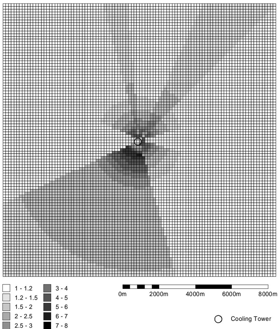
Figure 1. Amplification factors for the wind velocities between 5,5 and 6,9 m/s derived for a cooling tower of 175 m height
