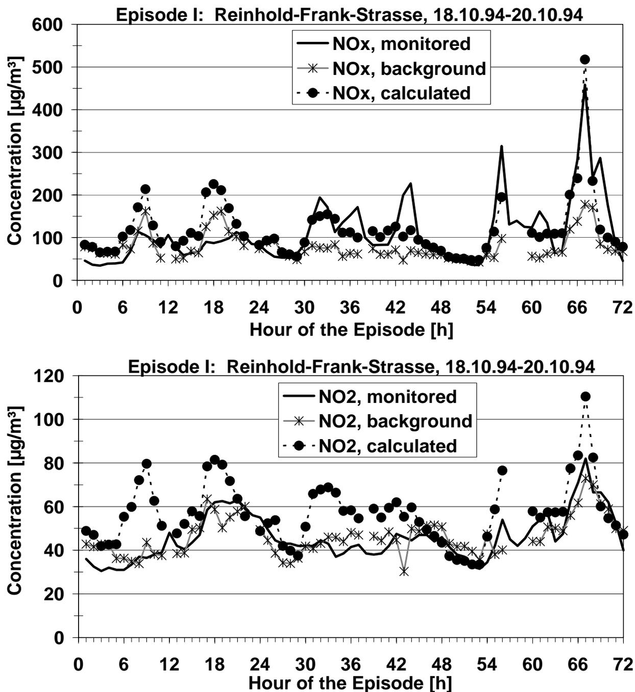
Figure 1. Comparison of monitored (in street canyon), calculated background and calculated (in street canyon)  $\text{NO}_x$  and  $\text{NO}_2$  concentrations for Episode 1.
