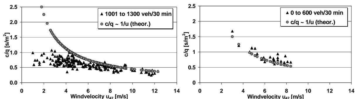
Figure 2. Thirty minute mean additional street canyon  $\text{NO}_x$  concentration  $c$  divided by source strength  $q$  as function of above roof wind speed ( $u_{42}$ ) for wind directions 250 to 270 degrees (perpendicular to street canyon axis). Left for hours with high traffic volume, right for low volume.
