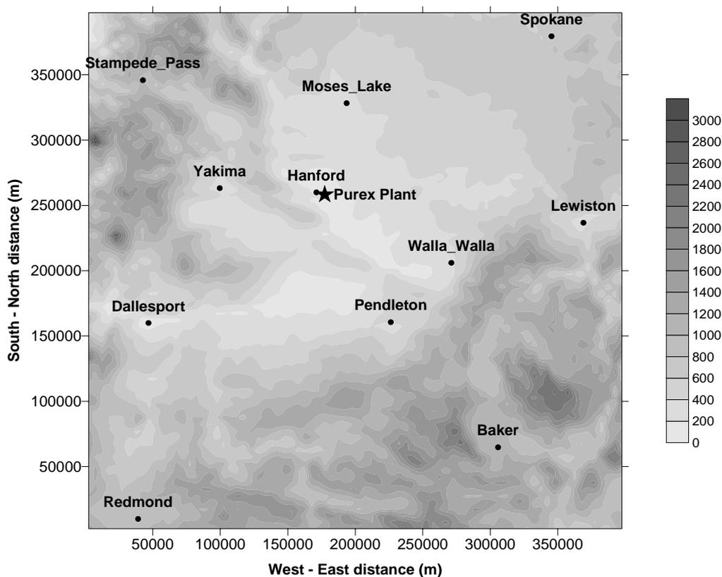
Figure 1. Computational domain for meteorology, with topography, the meteorological stations (dots) and the release location ("Purex Plant")
