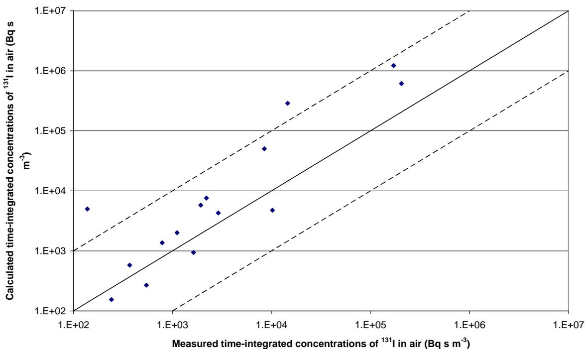
Figure 4. Scatter plot of calculated vs. observed time-integrated <sup>131</sup>I concentrations in air, for each day during the release and for all sensors with non-zero values. Factor-of-10 and 1:1 lines are also drawn
