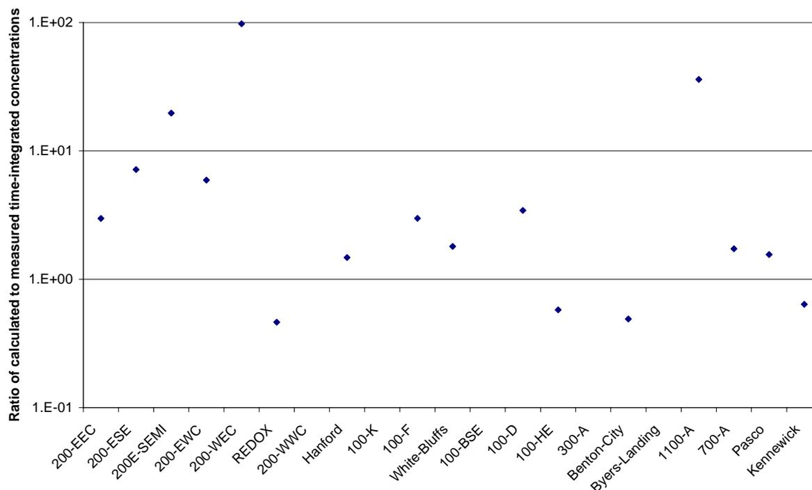
Figure 5. Ratio of calculated to observed time-integrated concentrations for the period of the release and for all sensors with non-zero values (ordered by increasing distance from the release point).
