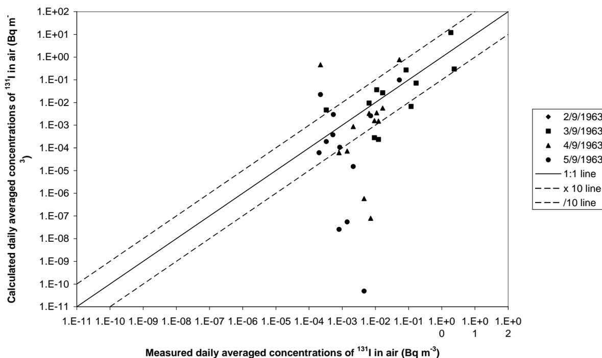
Figure 2. Scatter plot of calculated vs. observed  $^{131}\text{I}$  concentrations in air, for each day during the release and for all sensors with non-zero values. Factor-of-10 and 1:1 lines are also drawn.
