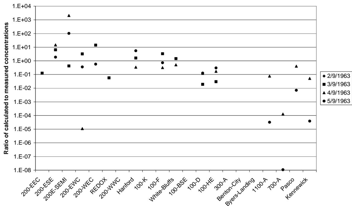
Figure 3. Ratio of calculated to observed daily averaged concentrations for all days of the release and for all sensors with non-zero values (ordered by increasing distance from the release point).
