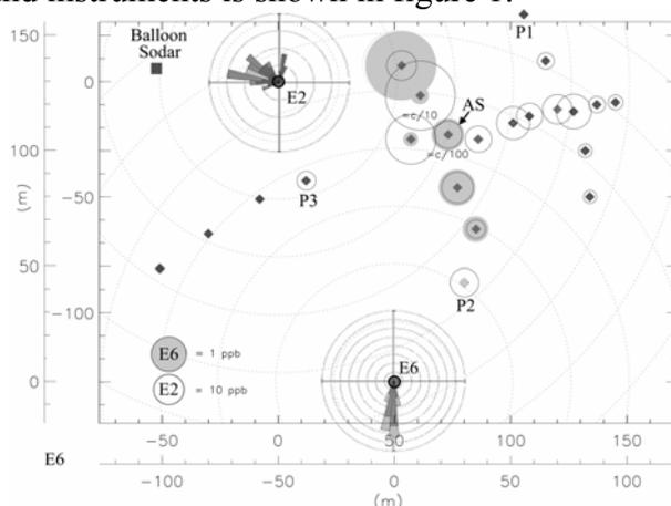
Figure 1. Schematic of setup and measured concentration fields of experiments E2 (white dots) and E6 (grey filled dots). Fractional concentrations refer to E6. Diamonds refer to tracer sampling stations. Axis are given with the point of origin being located at the release point. Additionally wind conditions at the release points are shown.
