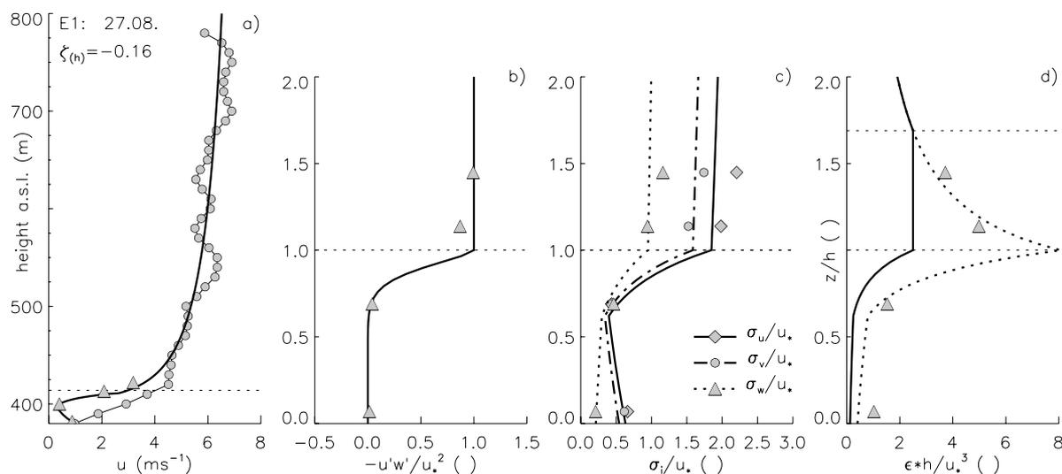
Figure 3. Integral statistics (30 min means) of the wind field. a) Mean wind profile: line stands for parameterisation, grey dots for tethered balloon and grey triangles for sonic measurements. Normalised profiles of b) (kinematic) momentum flux c) standard deviations and d) dissipation rate. Lines stand for parameterisations, symbols for sonic measurements. In d) the solid line stands for a parameterisation considering a roughness sublayer.
