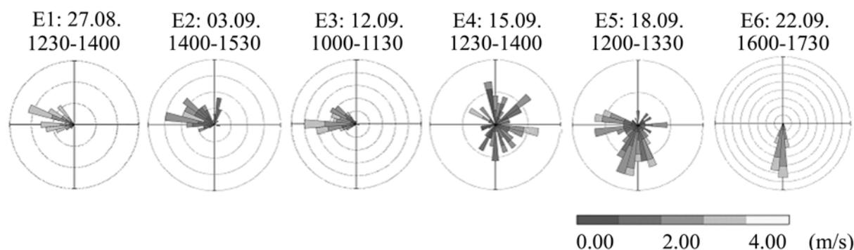
Figure 2. Frequency distribution of wind direction and speed basing on 1 min mean data measured in trunk space. Times indicated are given in CET (=GMT+1).
