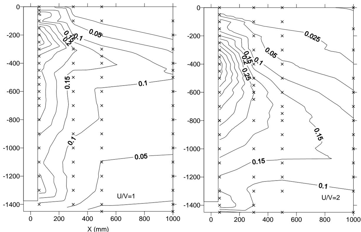
Figure 4. Concentration field at the ground downwind of the street –  $90^\circ$
