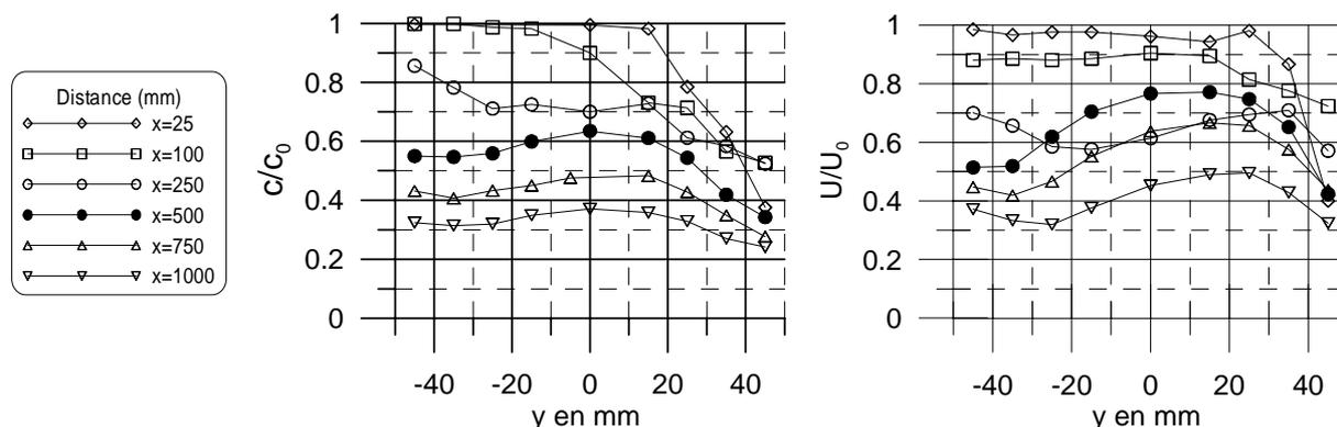
Figure 3. Evolution of the flow in the street canyon according to the distance at the exit – Profile at half-height of the street for  $90^\circ$  and a ratio of 0.5.
