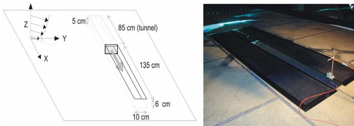
Figure 1. Small-scale model
