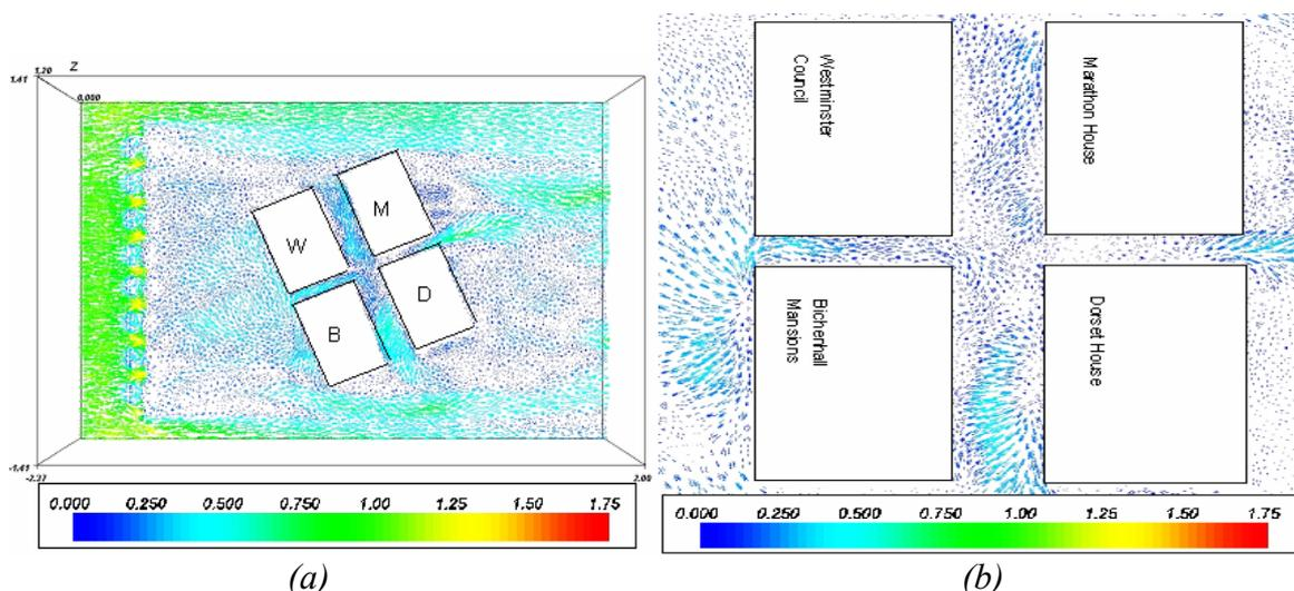
Figure 2. (a) Wind velocity distribution on the plane  $z=H/2$ ,  $t = 510s$ ; (b)  $z=H/7.5$ ,  $t = 510s$
