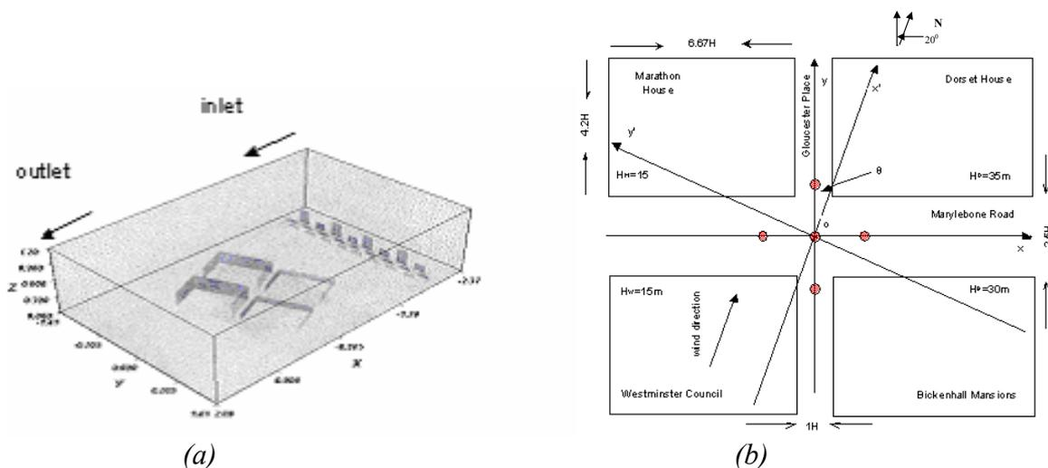
Figure 1. (a) Computational domain, mesh at 510s full-scale time. (b) Plan of model arrangements and coordinate axes. The red filled circles are detectors to record time series of variables.  $x'$ ,  $y'$  are axis used in LES computation, whereas  $x$  and  $y$  system are adopted to discuss the results. The streets are named according to the initial letters of the buildings alongside, e.g. W-M runs between Westminster Council House and Marathon House.
