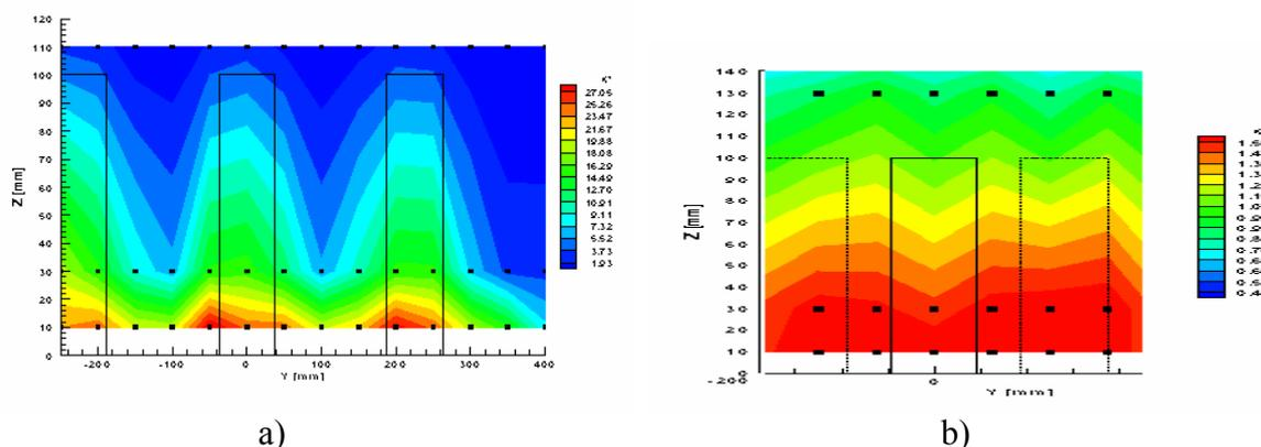
Figure 2. Mean concentration spread within the canopy layer behind the linen source a)  $x/S_x = 0,1$  b)  $x/S_x = 1,1$  (Here  $S_x$  denotes roughness element spacing,  $x=0$  for linen source and rectangles denote the roughness elements).
