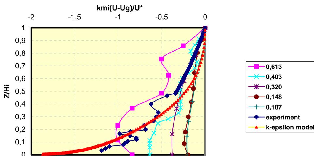
Figure 1. Comparison of velocity defect profiles inside the UABL simulations with radio sounding launched in Barcelona and wind tunnel experiment. (Number denotes the value of  $\mu$ )
