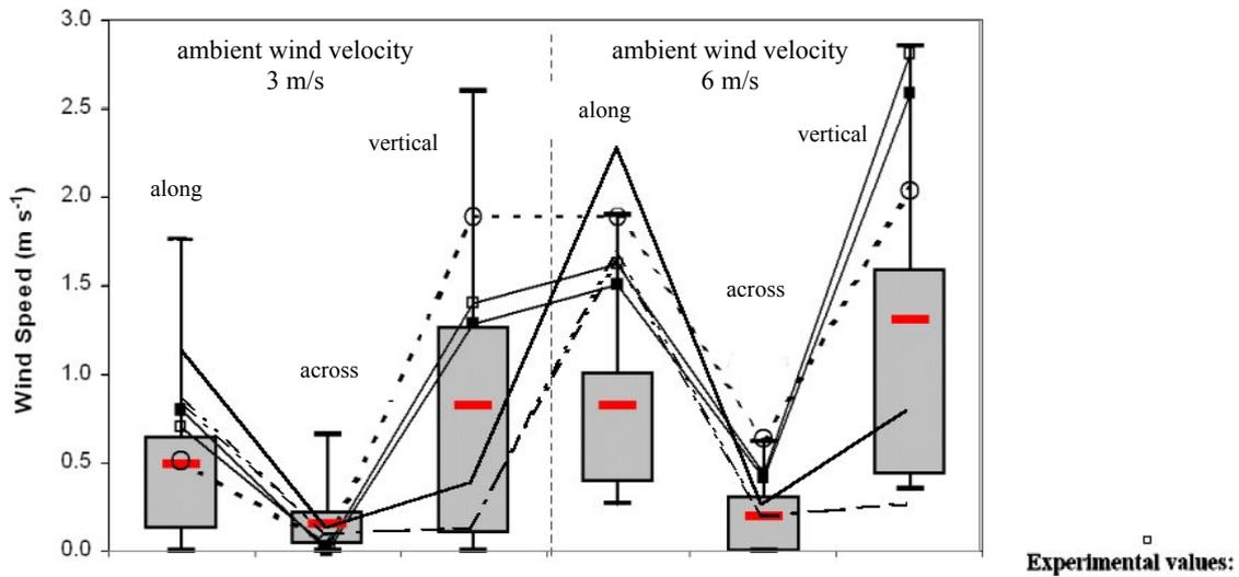
Figure 3. Comparison of velocity components results obtained for oblique flow
