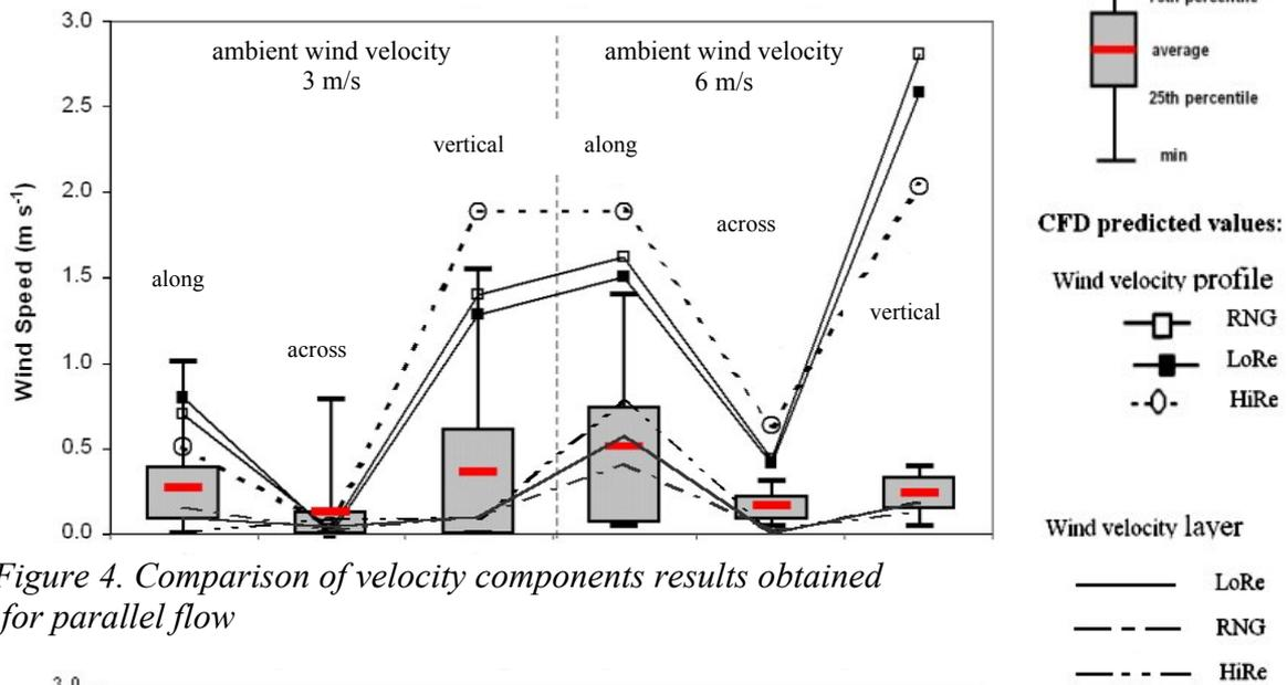
Figure 4. Comparison of velocity components results obtained for parallel flow
