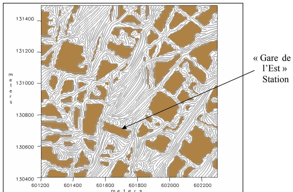
Figure 2. Streamline for South western wind 5m/s
