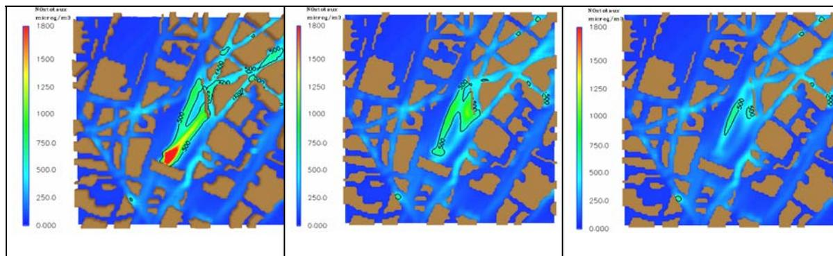
Figure 5. Impact on air quality 6 minutes after engine starts: from left to right, 1) old engines 2) new warming up protocol (reduced from 6 to 2 minutes) 3) new motorization of engines.
