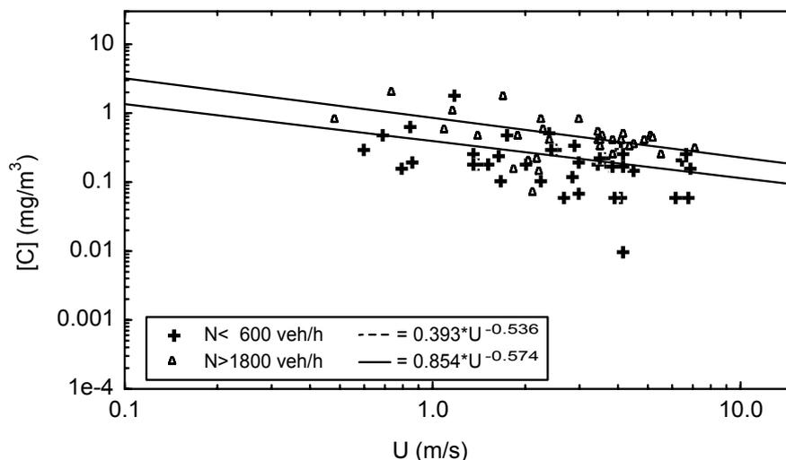
Figure 1. Local CO concentration  $[C=C_i$  (inside the street canyon)- $C_b$ (background)] versus wind speed for two traffic flows. Windward conditions.
