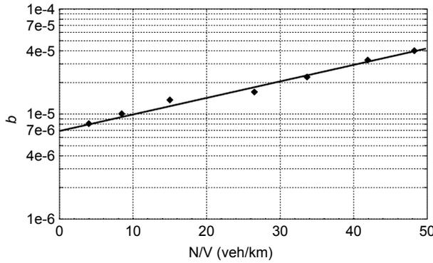
Figure 3. Variation of b (Eq.(1)) with traffic density (N/V). The line shows the best fit [Eq.(3)]
