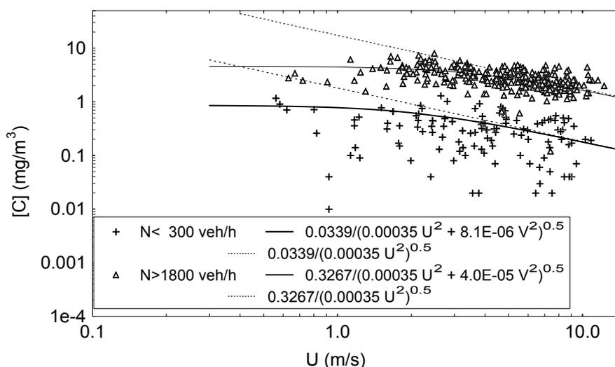
Figure 2. Local CO concentration  $[C=C_i$  (inside the street canyon)- $C_b$ (background)] versus wind speed for two traffic flows. Leeward conditions.
