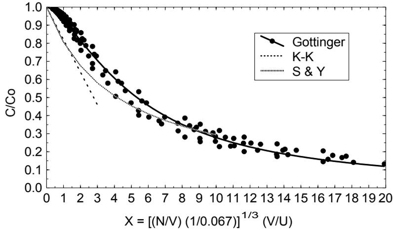
Figure 5. Influence of TPT. Comparison of on site results (Göttinger Strasse) with wind tunnel result (K-K) and model simulation (S&Y). See text for further explanations.
