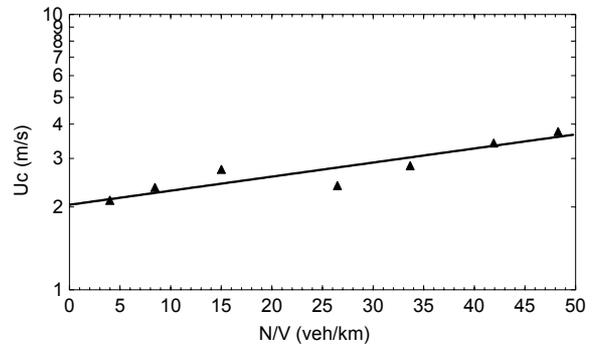
Figure 7. Variation of critical wind speed with traffic density. The line shows the best fit [Eq.(5)]
