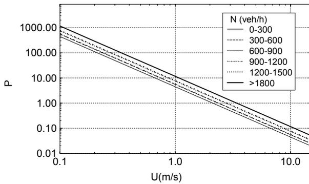
Figure 6. Calculated ratio  $P = aU^2/bV^2$ , as function of wind speed, for different traffic flows.
