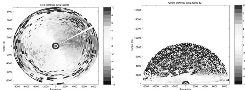
Figure 2. (left) showing a typical 'Azimuth Scan', by moving around a vertical axis, with flow from a south west direction. Figure 3 (right) shows a vertical scan with height vertical, range radial, and a rural to urban difference clearly evident.
