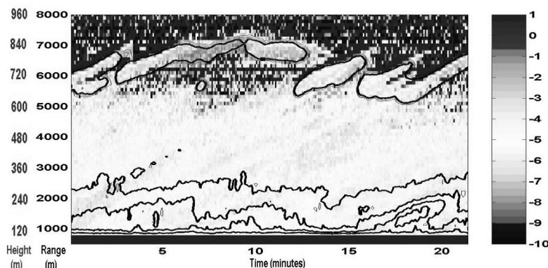
Figure 1. A 'Stand and Stare' plot, rather like a time series plot, colour coded for velocity with added contours indicative of intensity (aerosol number).
