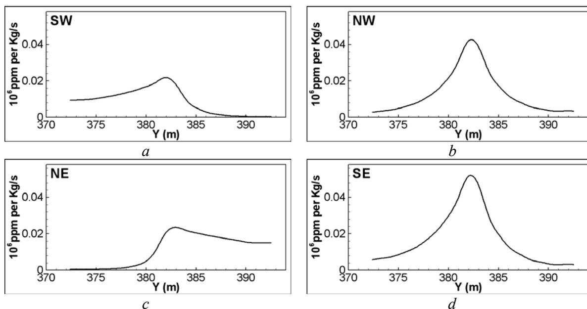
Figure 3. Concentration across the street for four wind directions.
