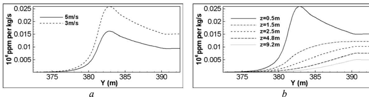
Figure 4. North wind concentration results. (a) Comparison of pollution levels for two different wind speeds at  $z=0.5\text{m}$  across the centre of the street canyon. (b) Different heights' concentration for the 3m/s wind speed case.
