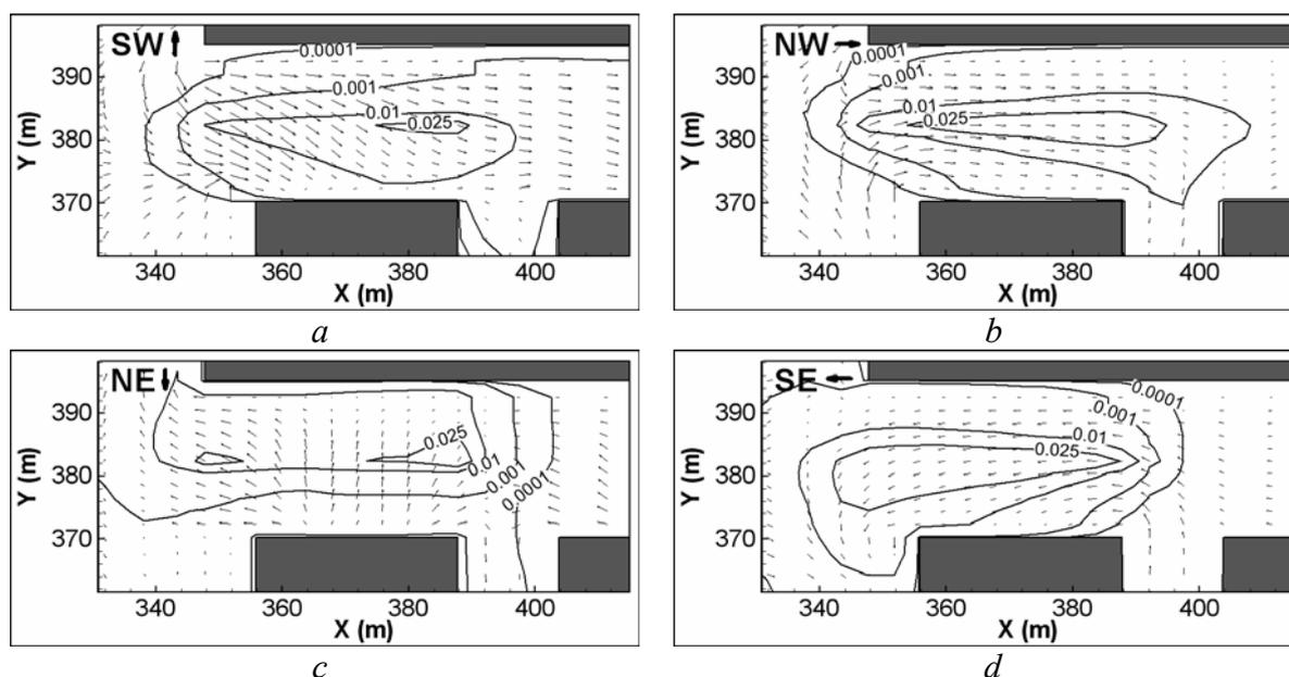
Figure 2. Concentration and flow field for SW (a), NW (b), NE (c) and SE (d) free wind stream directions. Contours for  $10^6$  ppm per kg/s of emission are presented at  $z=0.5$ m.
