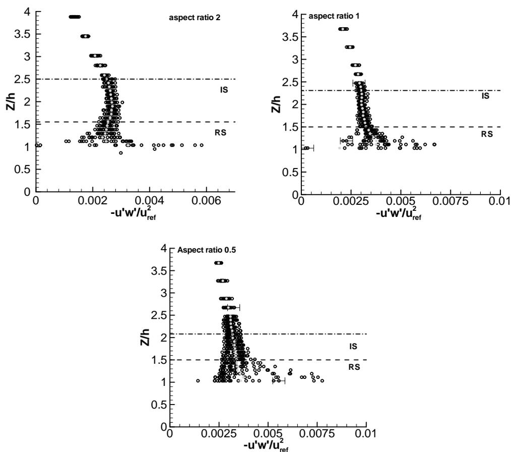
Figure 5. Normalised turbulent fluxes measured behind a fetch of 32 rows for cube arrays with aspect ratios varying from 0.5 to 2. Error bars indicate reproducibility.
