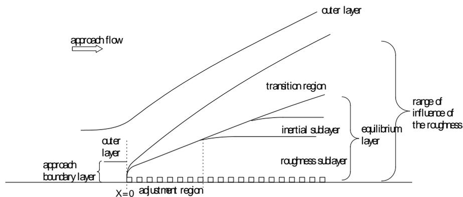
*Figure 3. Sketch of the flow development after a step change of roughness. (From Cheng and Castro, 2002).*
