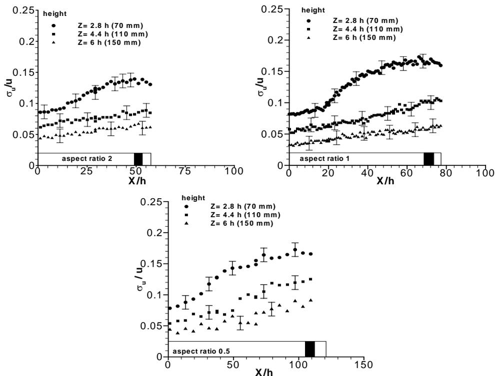
*Figure 4. Development of the longitudinal turbulent intensity  $\sigma_u/u$  with distance and height for cubes with identical height but different spacing (aspect ratios vary from 0.5 to 2).*
