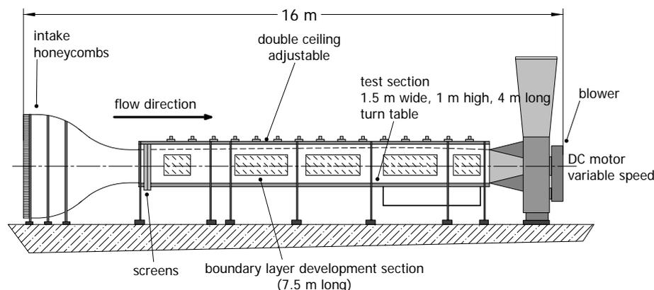
Figure 1. Sketch of the boundary layer wind tunnel “Blasius” at the Meteorological Institute of Hamburg University.
