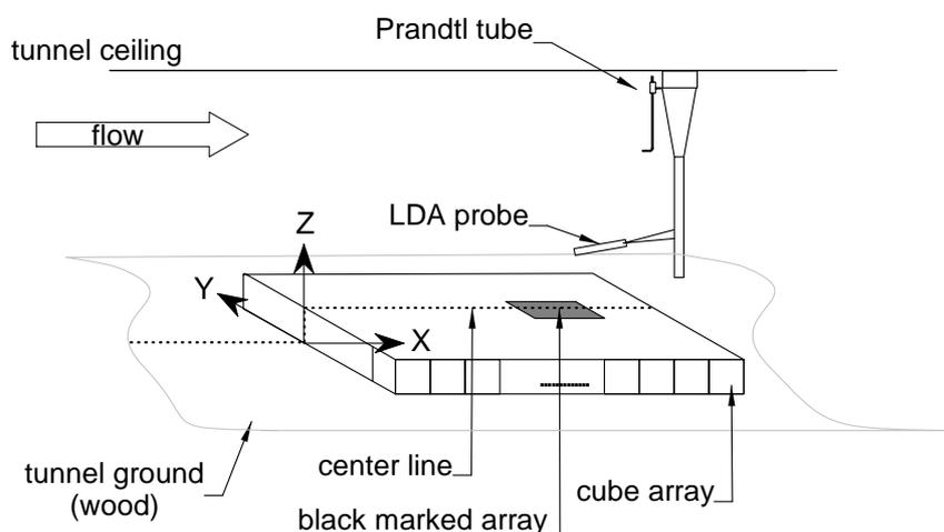
*Figure 2. Sketch of the experimental set-up in the wind tunnel.*
