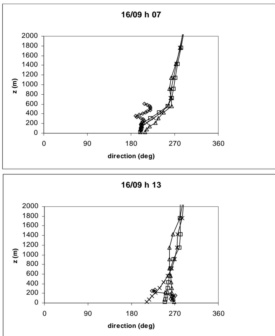
Figure 2: Velocity direction vertical profiles from Sodar measures (diamonds), M&Y (squares), isotropic E-l (triangles), E-l with horizontal deformation (crosses) models.
