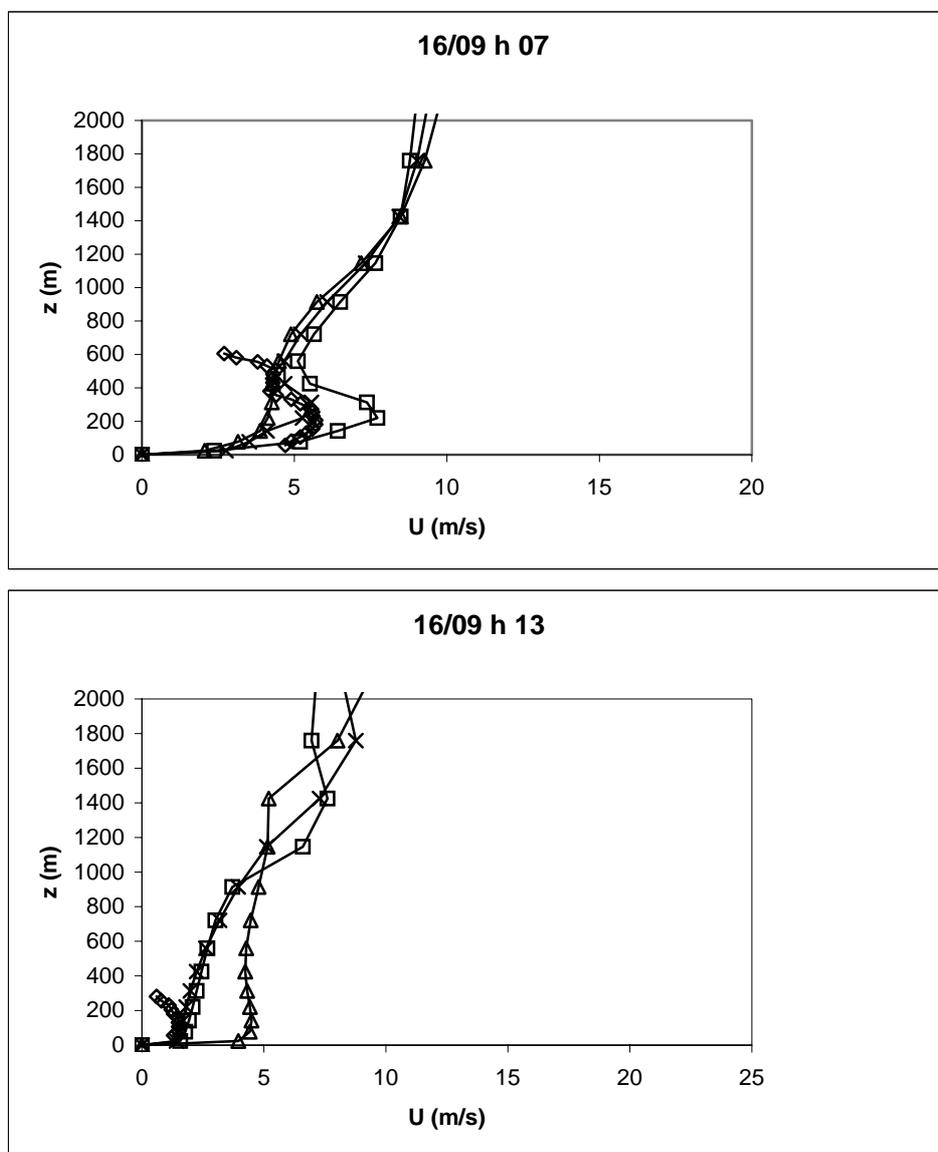
Figure 1: Velocity vertical profiles from Sodar measures (diamonds), M&Y (squares), isotropic E-l (triangles), E-l with horizontal deformation (crosses) models
