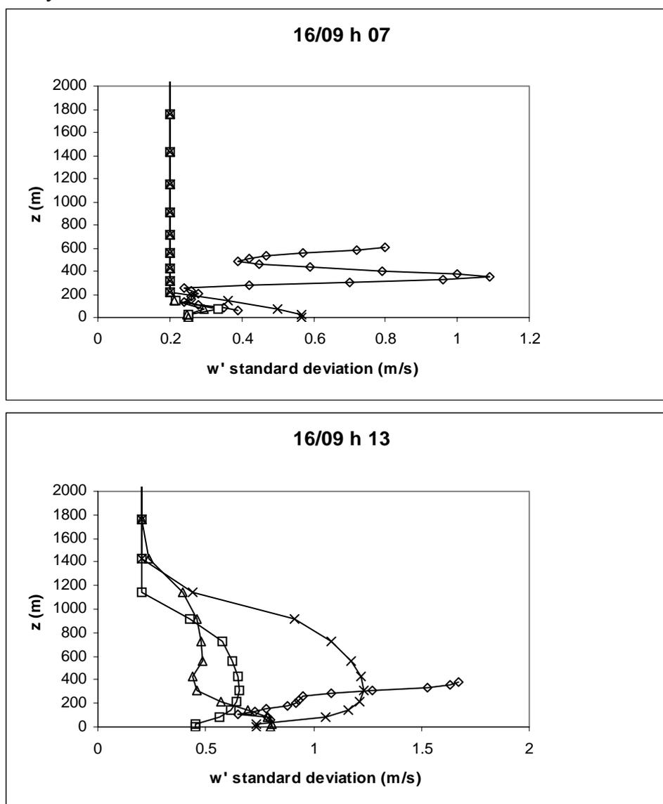
Figure 3:  $w'$  standard deviation vertical profiles from Sodar measures (diamonds), M&Y (squares), isotropic E-l (triangles), E-l with horizontal deformation (crosses) models.
