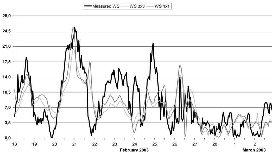
Figure 2. Comparison of measured wind velocity ( $m.s^{-1}$ ) with TAPM simulations.
