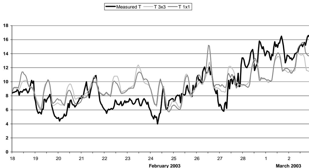
Figure 1. Comparison of measured surface temperature (°C) with TAPM simulations.
