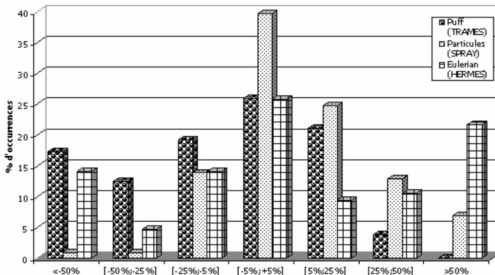
Figure 5. General score (all data) for this episode (bubbles: TRAMES puff model; dots : SPRAY Lagrangian model; grid: HERMES Eulerian model). Along X : error range class, along Y : percentage of pair of computed and measured values falling in the range for each model.
