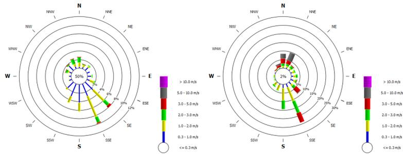
Figure 6. Relatively good correlation between measured and forecasted wind in the Šaleška region for the February 2011 (left: measured wind at 10 m station Ugreznine, right: forecasted wind by WRF).
