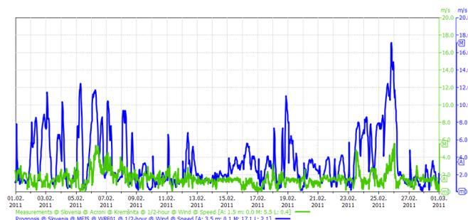
Figure 9. Comparison of wind speed for Jesenice region for the February 2011 between measured wind at 10m, station Kremšnica and forecasted wind by WRF
