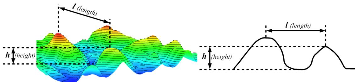
Figure 1. Illustration of the hLTc (height and length of Topographic complexity) index (left: figure presents dimensions in 3D view of topography, right: figures presents dimensions in vertical cross-section).
