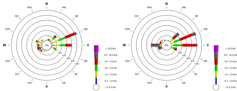
Figure 4. Excellent correlation between measured and forecasted wind in the Posavje region for the February 2011 (left: measured wind at meteorological tower on 70m near nuclear power plant, right: forecasted wind by WRF).
