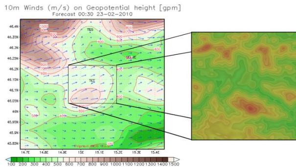
Figure 2. Zasavje region and its surroundings as seen by WRF model (left) in 4km horizontal resolution and the inner domain of 20 km by 20 km as seen by Swift model in 0.2 km horizontal resolution.
