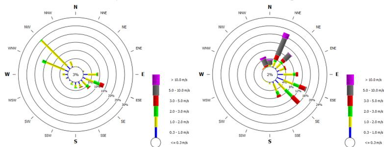
Figure 8. Relatively bad correlation between measured and forecasted wind for Jesenice region for the February 2011 (left: measured wind at 10m, station Kremšnita, right: forecasted wind by WRF)
