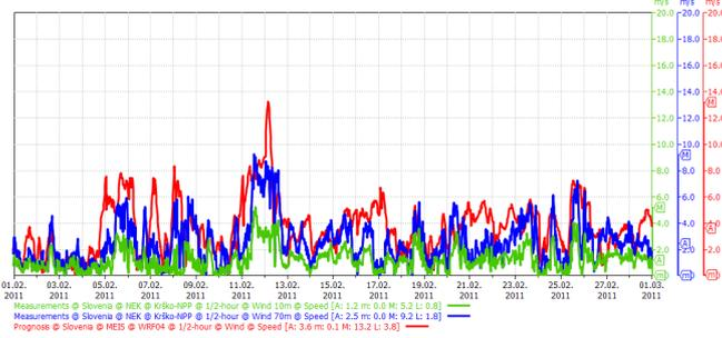
Figure 5. Wind for Posavje region is measured at the meteorological tower at heights 10 m, 40 m and 70 m. Comparison of wind speeds for the February 2011 as presented on the graph show that the correlation increases with the height. Comparison is made between measured wind at meteorological tower on two heights (10 m and 70 m) and forecasted wind by WRF (measured data from SNSA Data portal, 2011).
