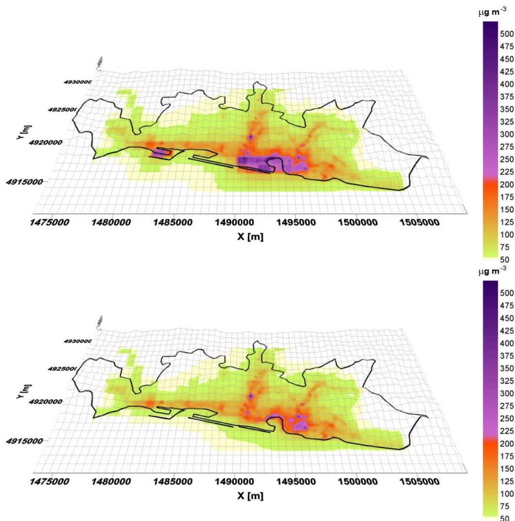
Figure 14. Concentration maps of NO<sub>x</sub> at 2m above the ground level for the year 2008, with harbour activities emissions (top) and without harbour activities emissions (bottom). Reported values are mean hourly concentrations obtained by the average of hourly values simulated for the whole period of simulation. Concentration values should be compared with the limit of 200 µg m<sup>-3</sup> fixed by European directive on air quality 2008/50.
