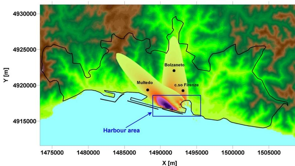
Figure 13. Test simulations with ADMS-Urban for the evaluation of the impact of harbour activities emissions on the urban area. Two cases are reported: one with SE wind of  $5 \text{ ms}^{-1}$  intensity and one with S wind of  $5 \text{ ms}^{-1}$  intensity. The pollutant simulated is  $\text{NO}_x$  with arbitrary emission rates. The black line indicates the administrative boundaries of the city of Genoa, the blue rectangle indicates the most emissive harbour area.
