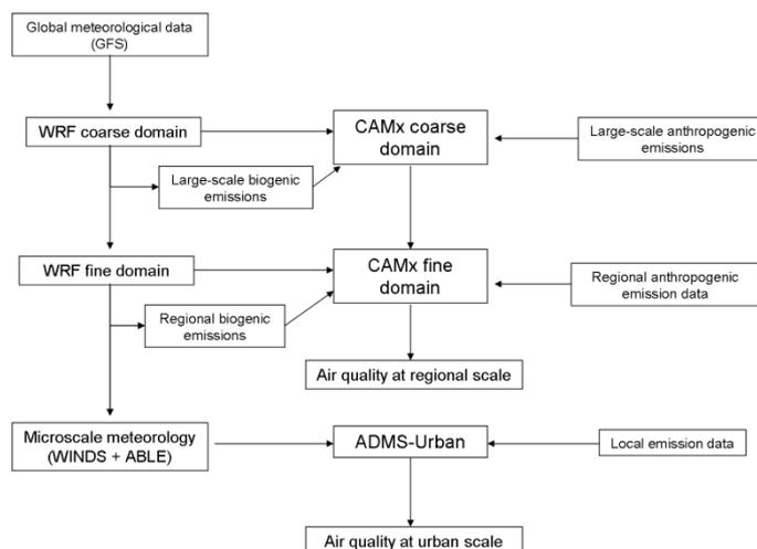
Figure 11. Simplified flow chart of the modelling system.
