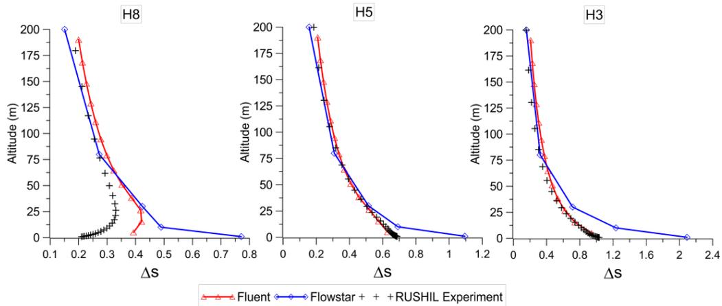
Figure 3 Profiles of speed-up for different steepness of the hills
