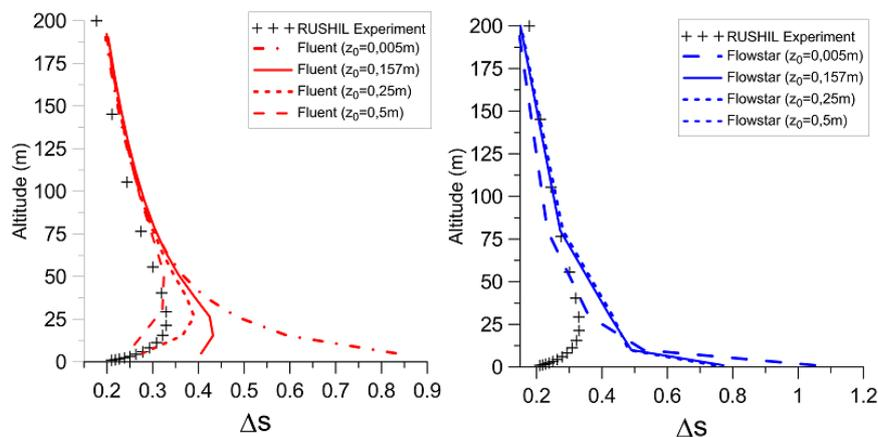
Figure 4 Profiles of speed-up for different roughness lengths for the H8 hill
