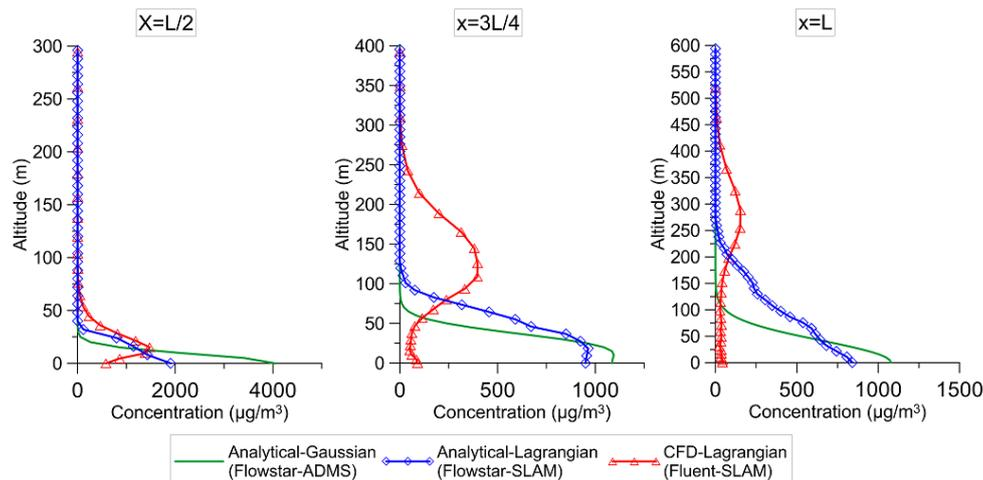
**Figure 6** Profiles of NO<sub>2</sub> concentrations at different locations, following the direction of the flow, in the presence of the Almeida single hill
