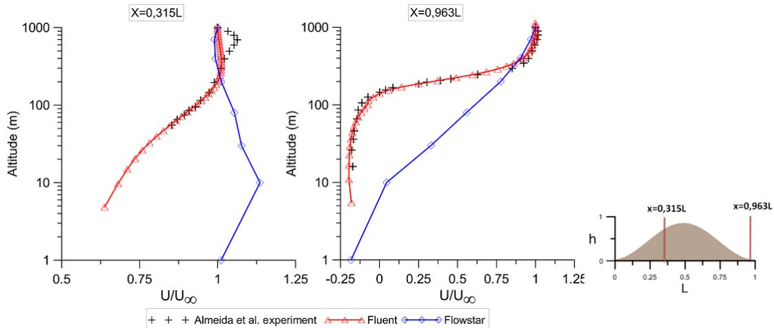
Figure 4 Profiles of horizontal wind velocity  $U$  for the single hill
