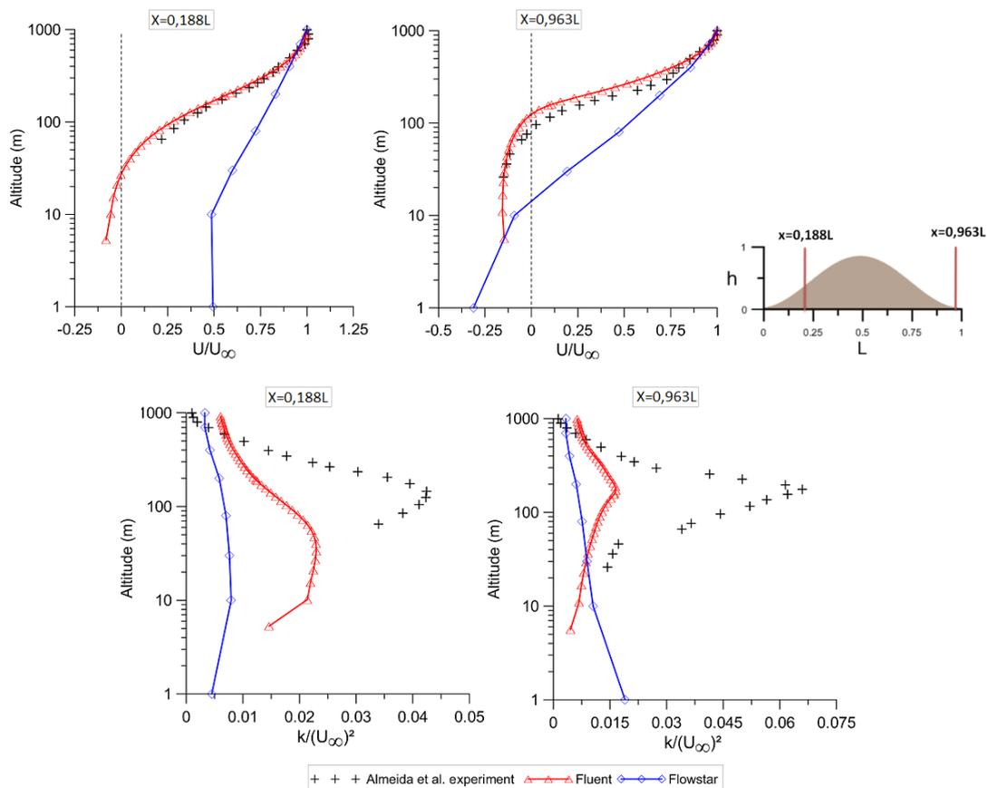
Figure 5 Profiles of horizontal wind velocity  $U$  and turbulent kinetic energy  $k$  for the multiple hills (between the third and the fourth hill)
