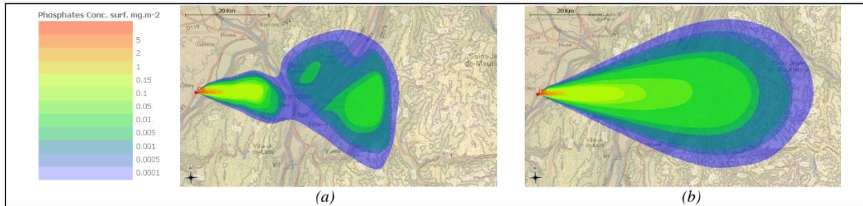
Fig. 22: Deposition ( $\text{mg.m}^{-2}$ ) of phosphate (a) taking into account relief, (b) without taking into account relief
