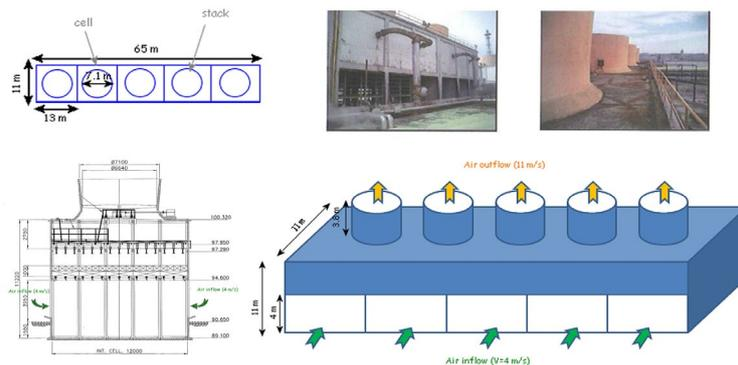
Figure 5. Details of the cooling towers
