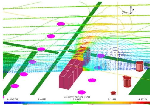
Figure 6. Velocity vectors on a section through the cooling towers
