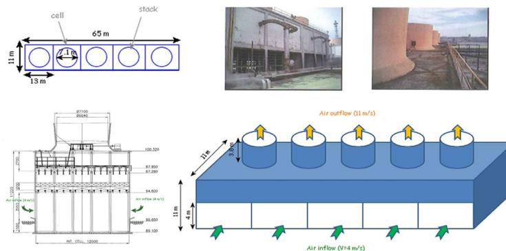
Figure 5. Details of the cooling towers
