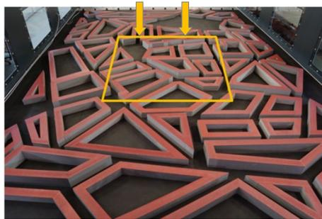
Figure 9. Wind-tunnel model of semi-idealized complexity. The rectangle encompassed the model region of densely spaced flow measurements. The arrows indicate the inflow direction.
